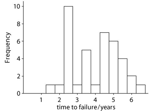
Fig. 3. Histogram of bearing failure times for 39 traction motors.
