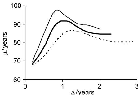
Fig. 6. For hybrid policy, MTBOF,  $\mu$ , against inspection interval,  $\Delta$ , for  $K = 3$  (— — — —),  $K = 4$  (—■—),  $K = 5$  (—●—).  $T = 10.248$ . Parameter values:  $p = 0.1, \eta_1 = 3, \eta_2 = 18, \beta_1 = 2.5, \beta_2 = 5, p = 0.1, \lambda = 1/2, C_R = 1, C_F = 10, C_I = 0.05$ . MTBOF calculated using simulation of 10,240 cycles.
