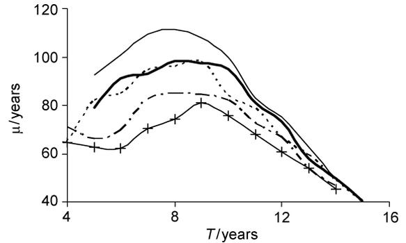
Fig. 7. For hybrid policy, MTBOF,  $\mu$ , against age at preventive replacement,  $T$ , for  $K = 1$  (—+—),  $K = 2$  (— — — —),  $K = 3$  (— — — —),  $K = 4$  (—■—),  $K = 5$  (—●—).  $\Delta = 0.861$ . Parameter values:  $p = 0.1, \eta_1 = 3, \eta_2 = 18, \beta_1 = 2.5, \beta_2 = 5, \lambda = 1/2, C_R = 1, C_F = 10, C_I = 0.05$ . MTBOF calculated using simulation of 10,240 cycles.
