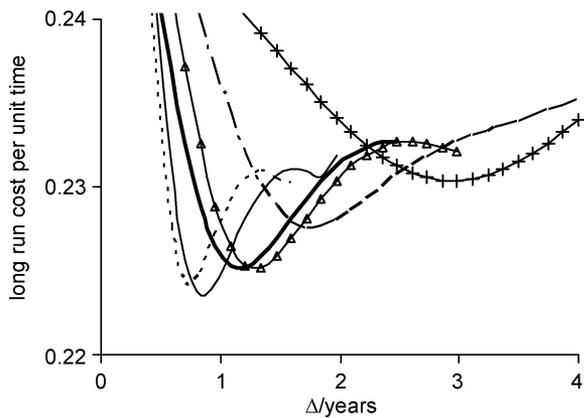
Fig. 5. Long run cost per unit time,  $C_\infty(T, \Delta, K)$ , as a function of inspection interval,  $\Delta$ , for  $K = 1$  (—+—),  $K = 2$  (— — — —),  $K = 3$  (— $\Delta$ —),  $K = 4$  (—■—),  $K = 5$  (—●—),  $K = 6$  (— — — —).  $T$  held at the optimum value specific for each value of  $K$  (for  $K = 5, T = 10.248$ ). Parameter values:  $p = 0.1, \eta_1 = 3, \eta_2 = 18, \beta_1 = 2.5, \beta_2 = 5, \lambda = 1/2, C_R = 1, C_F = 10, C_I = 0.05$ .
