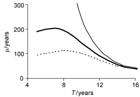
Fig. 8. For the hybrid policy, MTBOF,  $\mu$ , against age at preventive replacement,  $T$  (with  $\Delta = \Delta^* = 0.861, K = K^* = 5$ ) for various values of the mixing parameter,  $p$ , in the time to defect arrival distribution:  $p = 0$  (—);  $p = 0.05$  (—■—);  $p = 0.1$  (— — — —). Parameter values:  $\eta_1 = 3, \eta_2 = 18, \beta_1 = 2.5, \beta_2 = 5, \lambda = 1/2, C_R = 1, C_F = 10, C_I = 0.05$ . MTBOF calculated using the approximation (6),  $\mu = E(V)/\rho$ .
