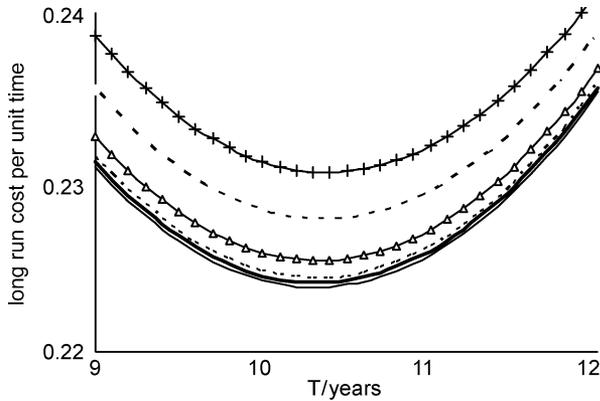
Fig. 4. Long run cost per unit time,  $C_\infty(T, \Delta, K)$ , as a function of age at preventive replacement,  $T$ , for  $K = 1$  (—+—),  $K = 2$  (— — — —),  $K = 3$  (— $\Delta$ —),  $K = 4$  (—■—),  $K = 5$  (—●—),  $K = 6$  (— — — —).  $\Delta = \Delta^* = 0.86$ . Parameter values:  $p = 0.1, \eta_1 = 3, \eta_2 = 18, \beta_1 = 2.5, \beta_2 = 5, \lambda = 1/2, C_R = 1, C_F = 10, C_I = 0.05$ .
