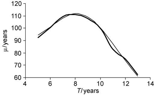
Fig. 10. For hybrid policy, MTBOF,  $\mu$ , against age at preventive replacement,  $T$  (with  $\Delta = 0.861$ ,  $K = 5$ ) for two cases: MTBOF calculated by simulation (—); MTBOF calculated using the approximation (6),  $\mu = E(V)/\rho$  (—). Parameter values:  $p = 0.1$ ,  $\eta_1 = 3$ ,  $\eta_2 = 18$ ,  $\beta_1 = 2.5$ ,  $\beta_2 = 5$ ,  $\lambda = 1/2$ ,  $C_R = 1$ ,  $C_F = 10$ ,  $C_1 = 0.05$ .
