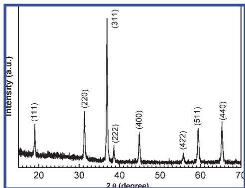
**Figure 1.** X-ray diffraction pattern of  $\text{Co}_3\text{O}_4$  nanorods.
