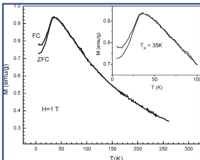
**Figure 5.** Temperature dependence of zero-field-cooled (ZFC) and field-cooled (FC) magnetic moment of  $\text{Co}_3\text{O}_4$  nanorods, measured in the field of 1 T. Inset: Details below 100 K, showing Néel temperature of 35 K.
