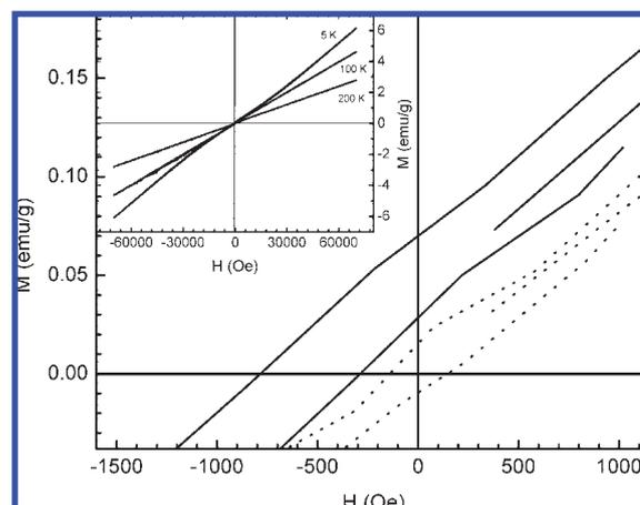
**Figure 6.** Magnetic hysteresis loops of  $\text{Co}_3\text{O}_4$  nanorods measured at 5, 100, and 200 K. The main figure shows the details around zero field for the hysteresis loops measured at 5 (solid line) and 100 K (dashed line).
