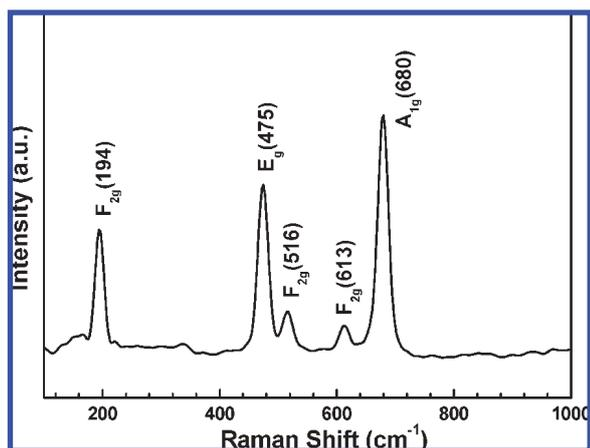
Figure 3. Room temperature Raman spectrum of  $\text{Co}_3\text{O}_4$  nanorods.
