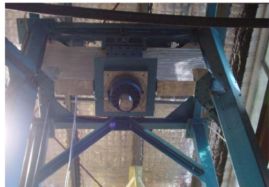
Figure 1 Main structure of the drop hammer
