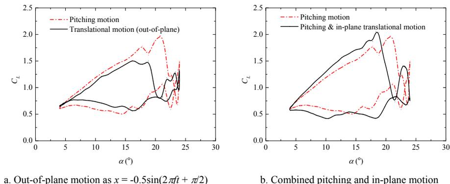
Fig. 3. Lift coefficients – pitching airfoil vs airfoil with translational motion
