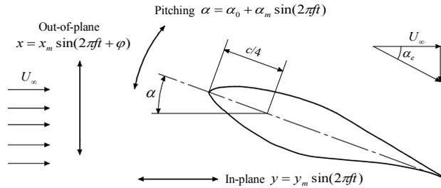
Fig. 1. Schematic of airfoil motion types
