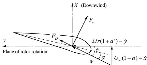
Fig. 4. Velocity diagram for a vibrating blade section
