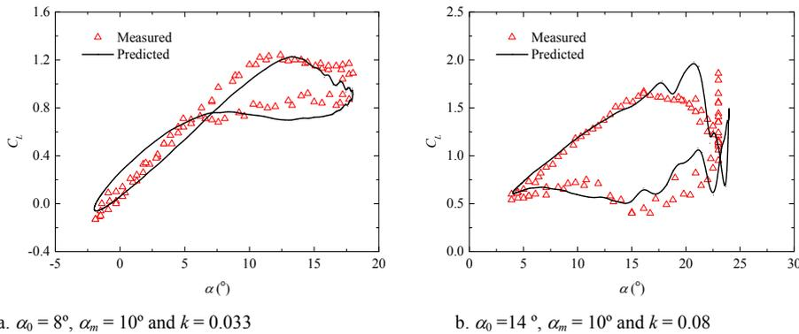
Fig. 2. Lift coefficients for pitching airfoil – predicted vs measured
