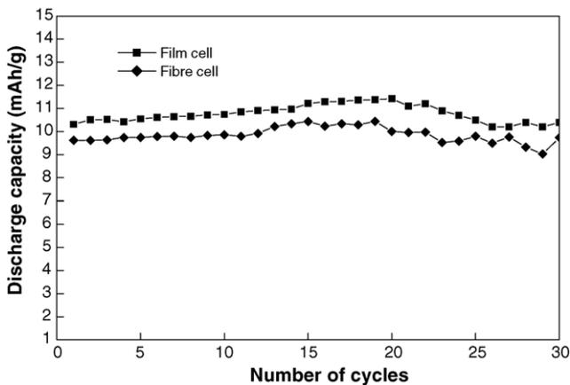
Fig. 7. Discharge capacity vs. cycle number for a fibre cell and a film cell of PPy/PF<sub>6</sub>|LiPF<sub>6</sub>–EC–DMC|PPy/PSS; current density = 0.1 mA h cm<sup>-2</sup>.
