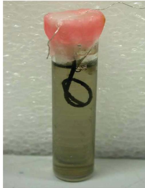
Fig. 8. Photograph of knotted fibre battery.
