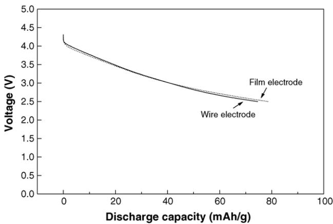
Fig. 4. Discharge curves obtained for PPY/PF<sub>6</sub>-coated Pt wire and film electrodes used as cathodes in lithium cell; current density = 0.1 mA h cm<sup>-2</sup>.
