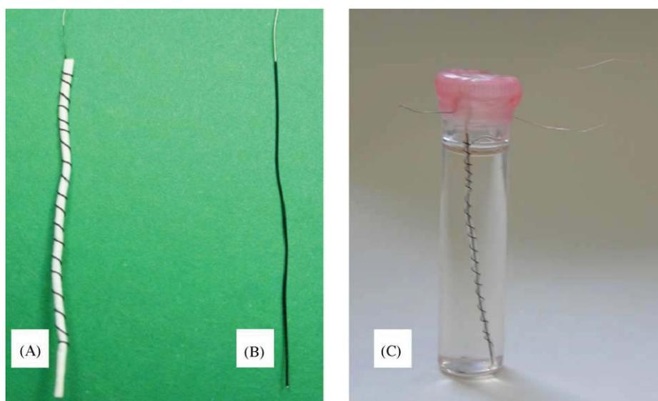
Fig. 3. Photographs of: (A) PPy/PSS/Pt wire–PVDF hollow fibre membrane composite anode; (B) PPy/PF<sub>6</sub>-coated Pt wire cathode; (C) test cell of PPy/PF<sub>6</sub> wire|LiPF<sub>6</sub>–EC–DMC|PPy/PSS–PVDF hollow fibre membrane composite.
