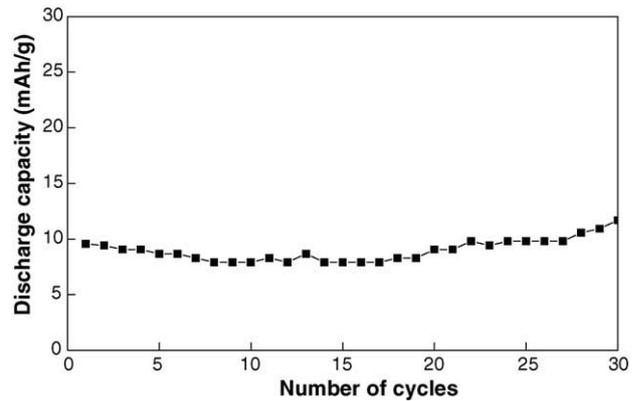
Fig. 9. Discharge capacity vs. cycle number of knotted fibre battery; current density = 0.1 mA h cm<sup>-2</sup>.
