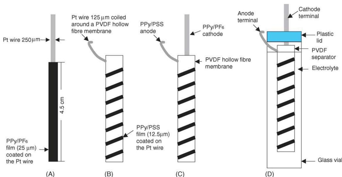
Fig. 2. Construction of hollow fibre composite cell. (A) PPy/PF<sub>6</sub>-coated Pt wire electrode; (B) PPy/PSS-coated Pt wire around PVDF hollow fibre membrane; (C) PPy/PF<sub>6</sub> cathode electrode inserted into PPy/PSS-coated Pt wire–PVDF hollow fibre membrane composite anode; (D) schematic of fibre cell.
