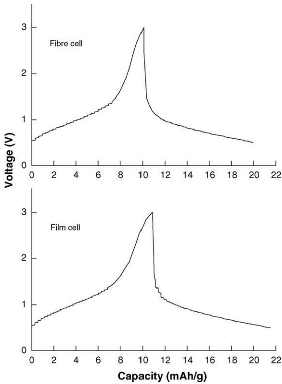
Fig. 6. Charge–discharge curves for fibre cell and film cell of PPy/LiPF<sub>6</sub>|LiPF<sub>6</sub>–EC–DMC|PPy/PSS; current density = 0.1 mA h cm<sup>-2</sup>.
