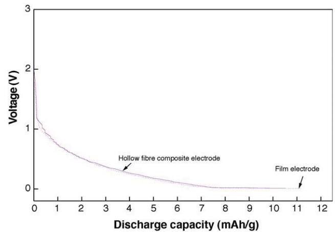
Fig. 5. Discharge curves obtained for PPy/PSS/Pt wire–PVDF hollow fibre membrane composite electrode and PPy/PSS film electrodes in lithium cells; current density = 0.1 mA h cm<sup>-2</sup>.
