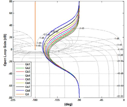
Fig. 2. Nichols plots of  $G(j\omega)$  function for different values of  $k_L$  in case of system operations without LG and Nichols plot of  $-1/N(A)$  (case-01).
