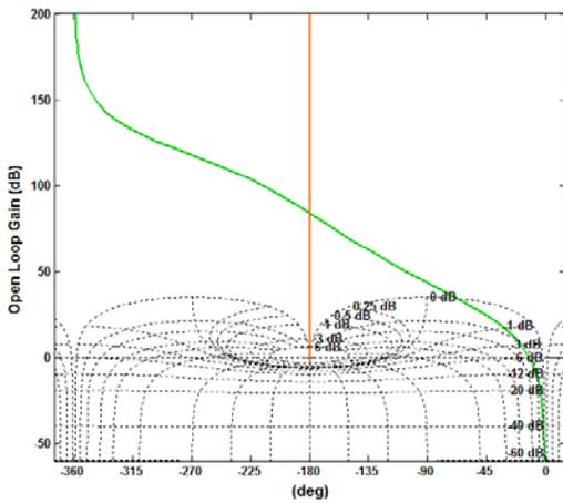
Fig. 9. Nichols plots of  $G(j\omega)$  for an existence of OLTC limit cycles in the multi bus system when  $k_L = 0.85$ ,  $P_{LG} = 34.6$  MW and  $Q_{LG} = 5.3$  MVar.
