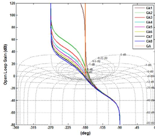
Fig. 5. Nichols plots of  $G(j\omega)$  function for different values of  $k_L$  in case of system operations with  $P_{LG} = 87.5$  MW (case-03).
