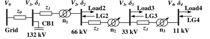
Fig. 12. Multi bus system model with cascaded OLTCs.
