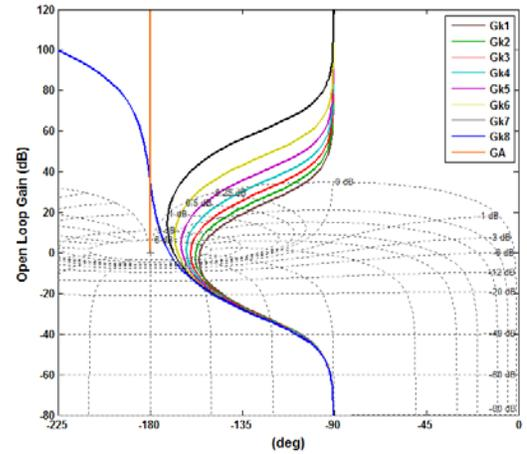
Fig. 7. Nichols plots of  $G(j\omega)$  function for different values of  $k_L$  in case of system operations with  $P_{LG} = 26.5$  MW and  $Q_{LG} = -9.6$  MVar (case-05).
