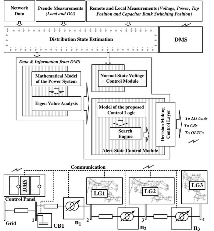
Fig. 11. Topology of the on-line implementation of proposed control strategy for an electricity network with cascaded OLTCs, CB and multiple LG units.
