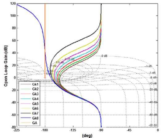
Fig. 3. Nichols plots of  $G(j\omega)$  function for different values of  $k_L$  in case of system operations with  $P_{LG} = 26.5$  MW (case-02).
