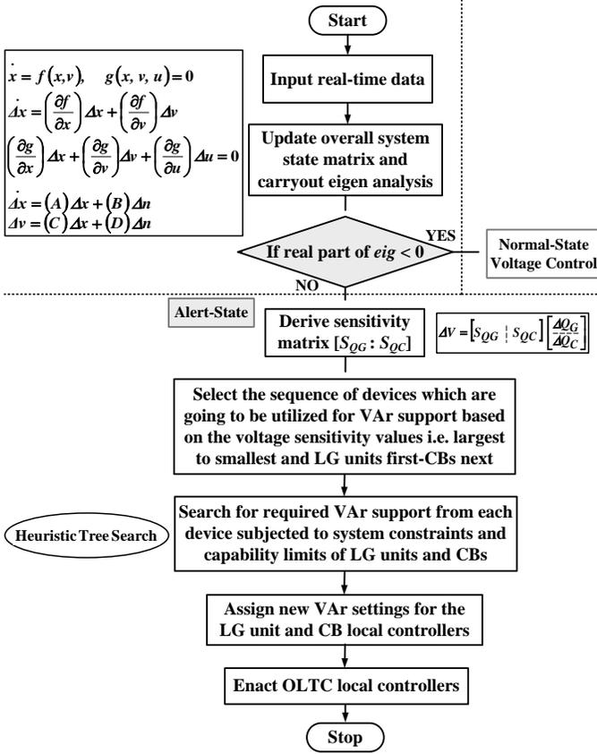
Fig. 10. Flow chart of the proposed voltage control algorithm with capability of mitigating OLTC limit cycles.
