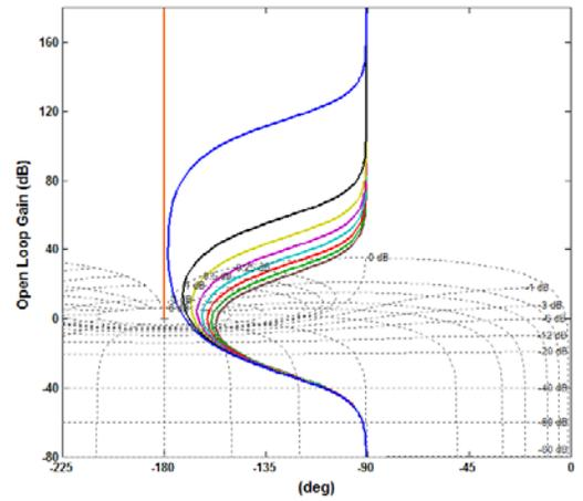
Fig. 6. Nichols plots of  $G(j\omega)$  function for different values of  $k_L$  in case of system operations with  $P_{LG} = 26.5$  MW and  $Q_{LG} = 13.5$  MVar (case-04).
