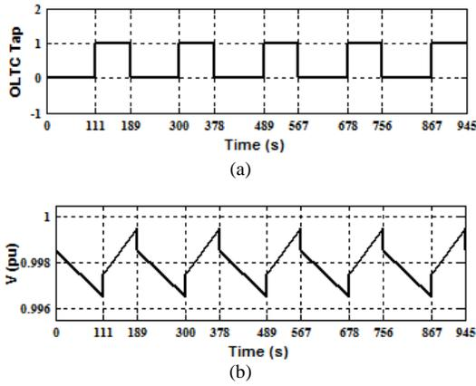
Fig. 4. Simulated (a) OLTC tap operations and (b) resultant voltage oscillations, which can occur due to OLTC limit cycle phenomenon predicted in case-02.
