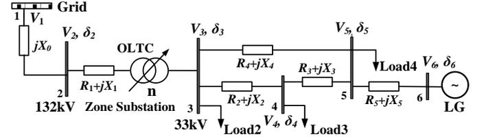
Fig. 8. Multi bus system model with single OLTC.
