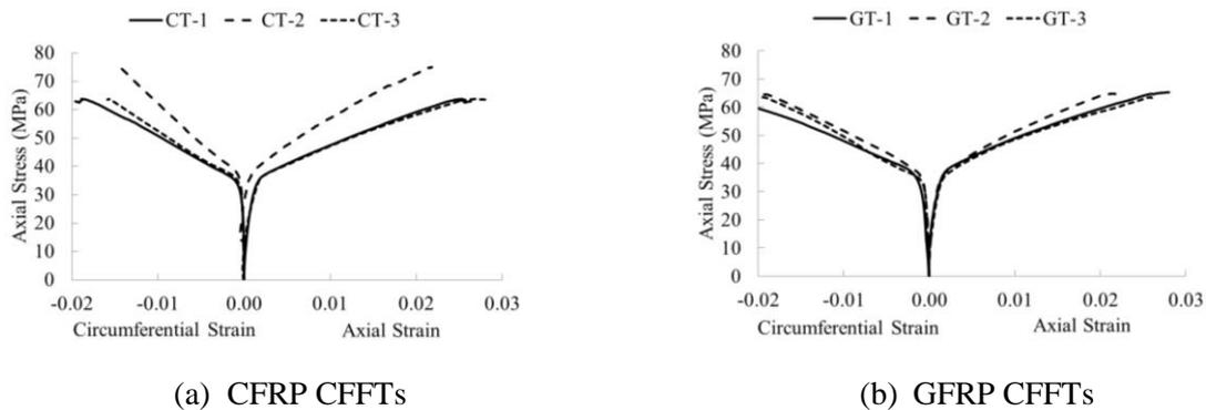
Figure 3: Axial stress-strain and axial stress-circumferential strain of circular CFFT specimens
