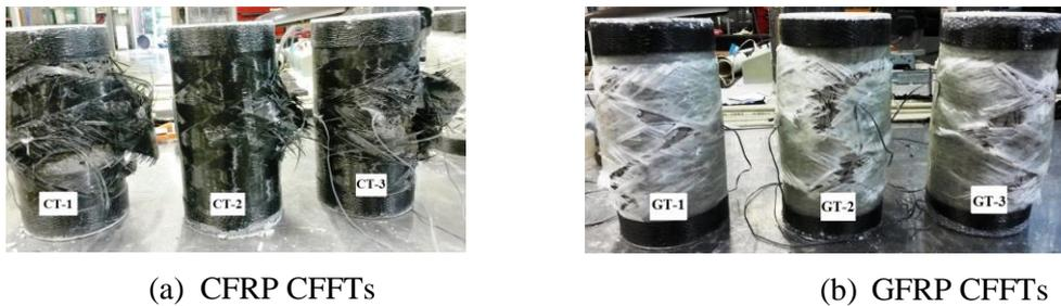
Figure 2 Observed failures in tested circular CFFT specimens
