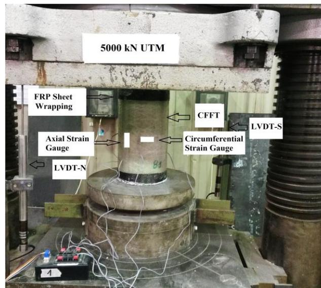
Figure 1 Axial compression testing arrangement
