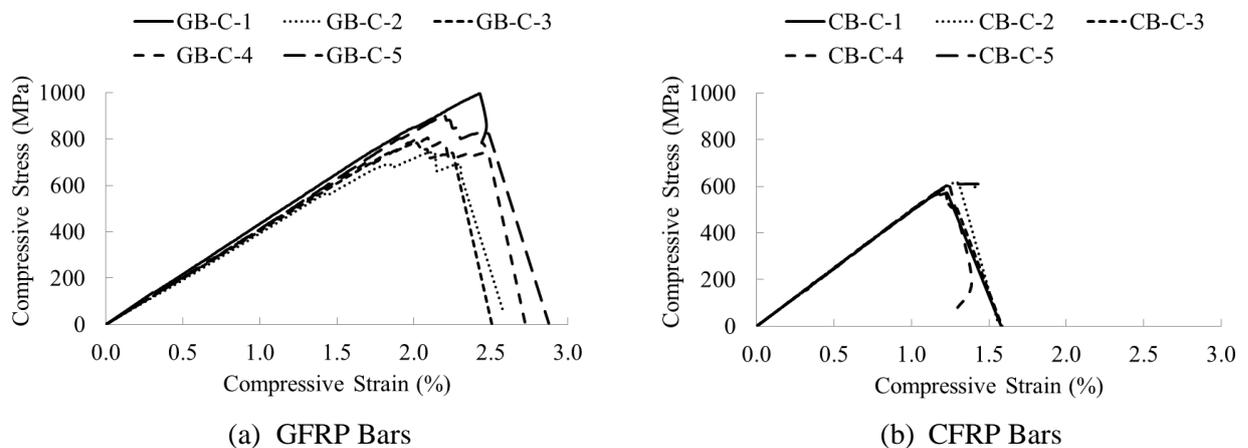
Figure 5 Compressive stress-strain of tested FRP bars
