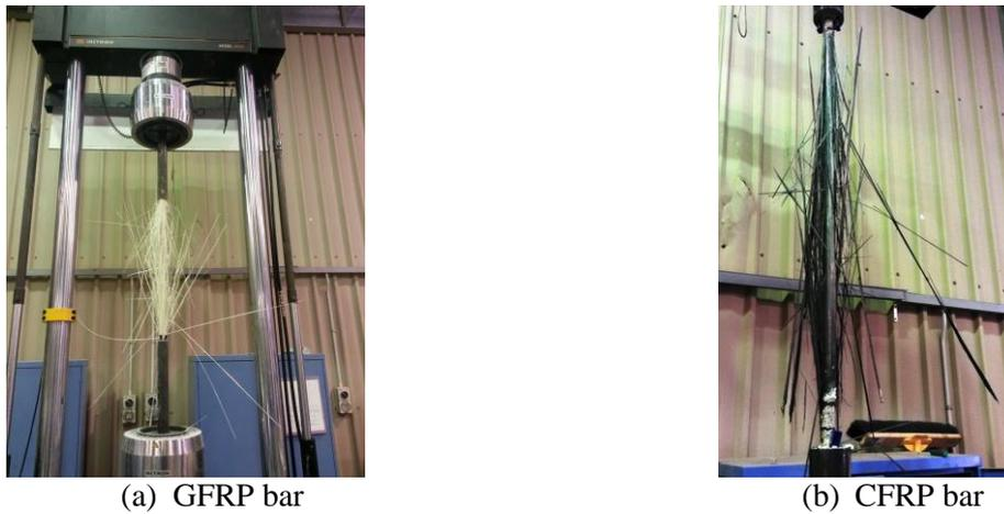
Figure 2 Observed tensile failure modes in tested FRP bars
