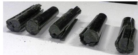
(b) CFRP bars
