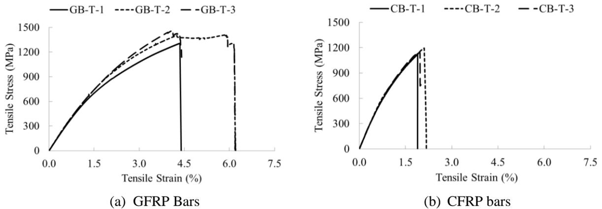
Figure 3 Tensile stress-strain in tested FRP bars
