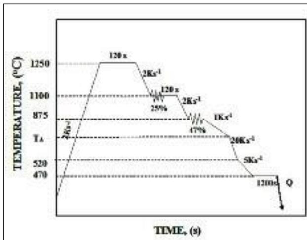
**FIG. 1** *Thermomechanical processing schedule.*
