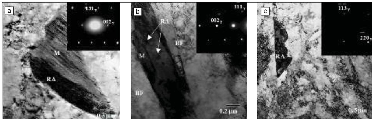
**FIG. 8** TEM micrographs of partial transformation of retained austenite to martensite at 0.02 strain, zone axis is  $[310]_{\gamma}$ , (a), partial transformation of retained austenite to martensite at 0.08 strain, zone axis is  $[110]_{\gamma}$ , (b) and retained austenite island after fracture, zone axis is  $[116]_{\gamma}$ , (c).
