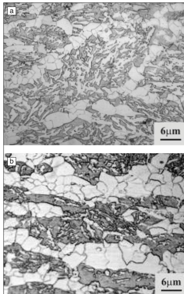
**FIG. 2** *Optical micrographs of Steel 1 (a) and Steel 2 (b).*
