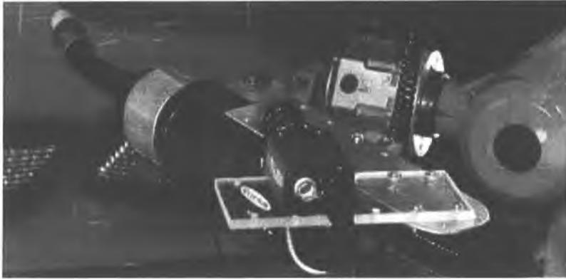
Figure 5. Touch sensing to determine workpiece profile
