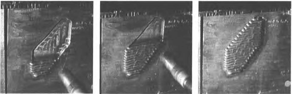
Figure 6. Deposit weld metal
