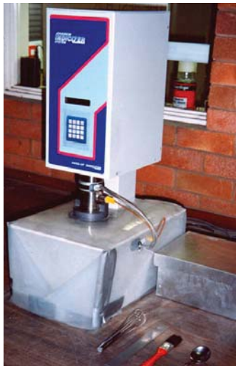
Fig 4 Johanson Hang-up Indicizer and Its Arrangement
