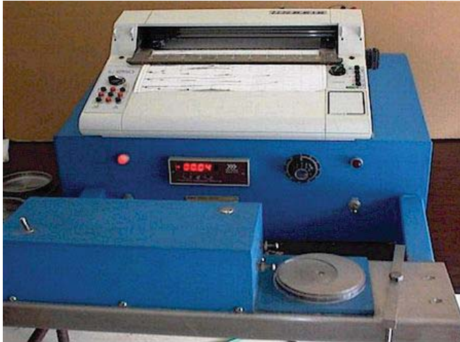
Fig 1 Jenike Direct Shear Tester
