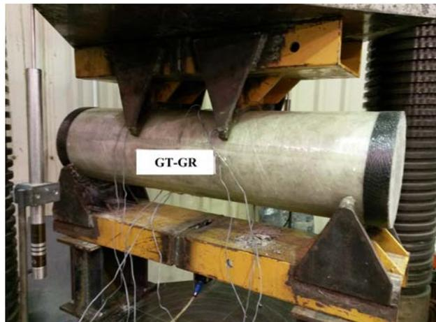
**Figure 1. Flexural testing arrangement used in this study**
