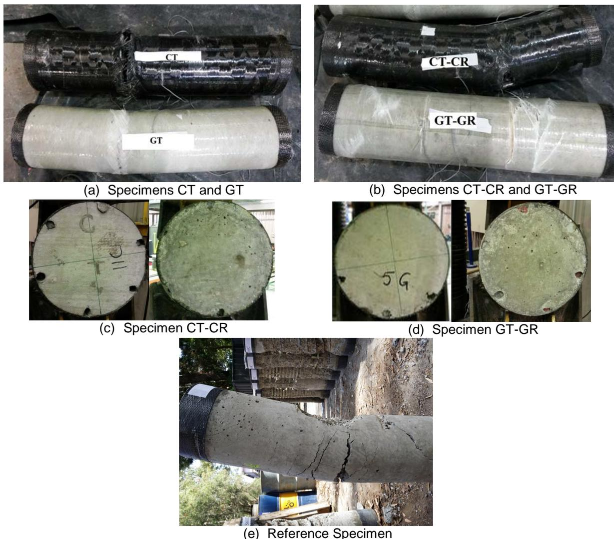
**Figure 2. Observed failure modes of the tested specimens**
