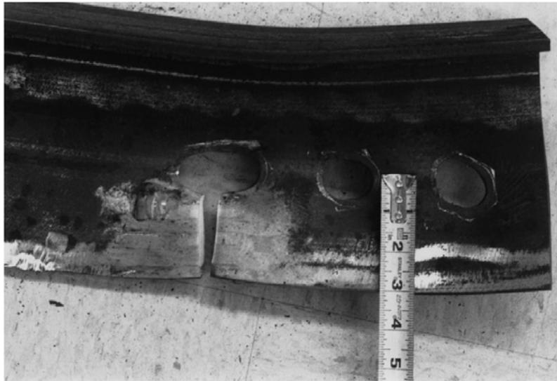
Figure 4 Tee section bolted at the web failing in block shear [10]
