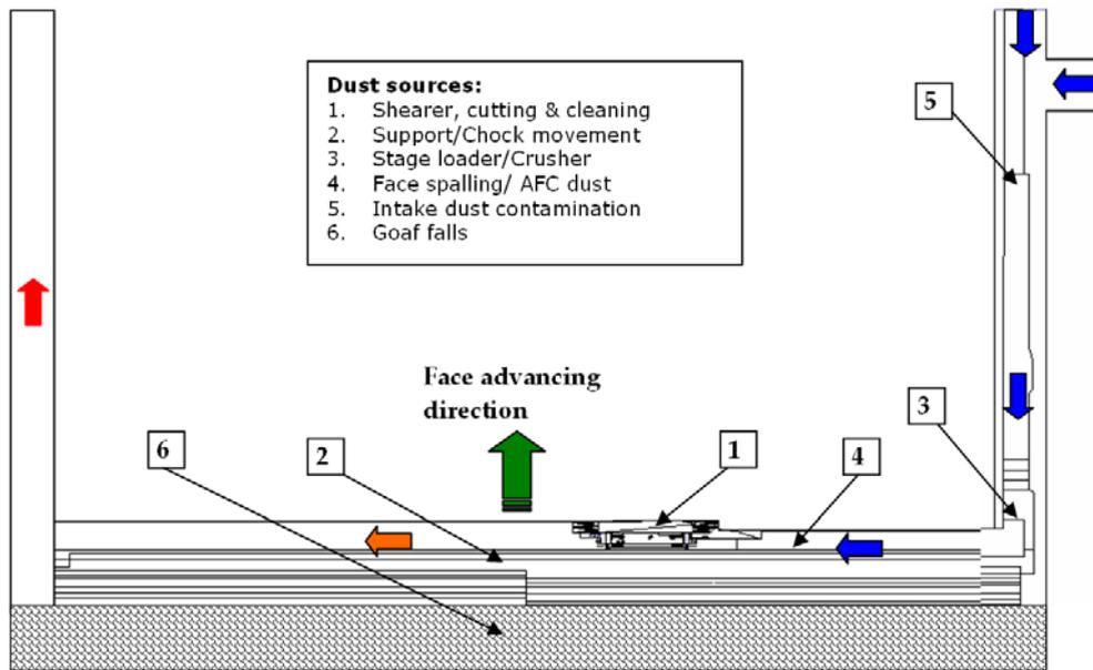
Fig.1. Main sources of dust generation on longwalls
