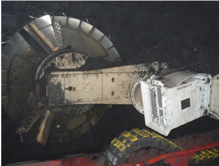
Fig.3. Dust scrubber installed on a longwall shearer
