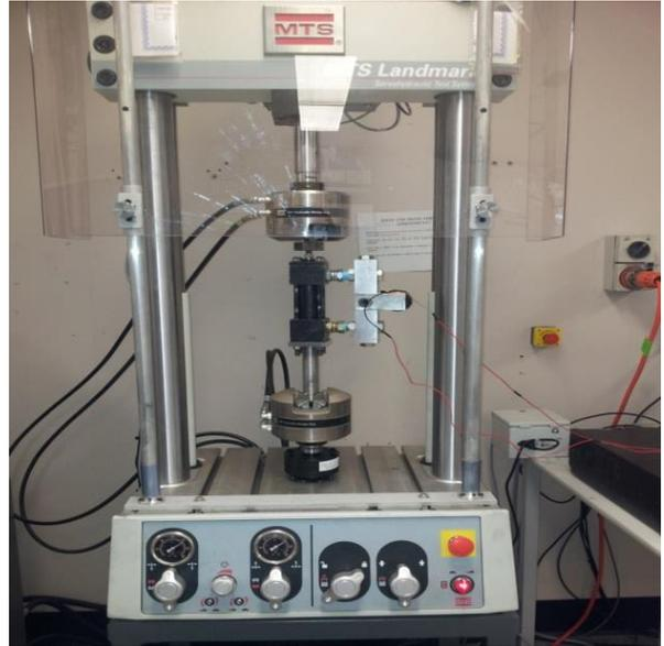
Fig. 2. MTS system for damper testing.
