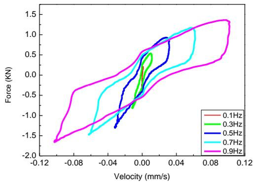
Fig. 6. ST effect of the 20% MRSTF filled damper.
