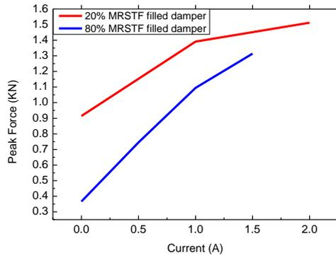
Fig. 8. Peak force versus current.
