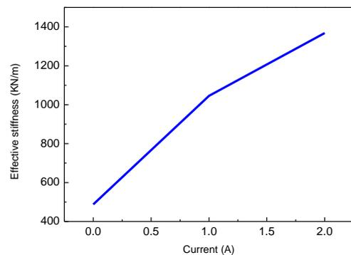
Fig. 5. Effective stiffness versus current
