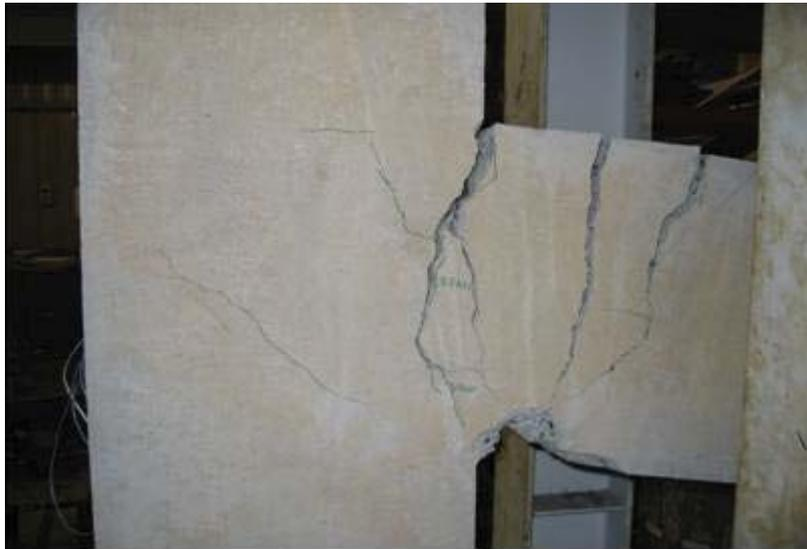
Figure 4 Cracks in damaged RC T-connection
