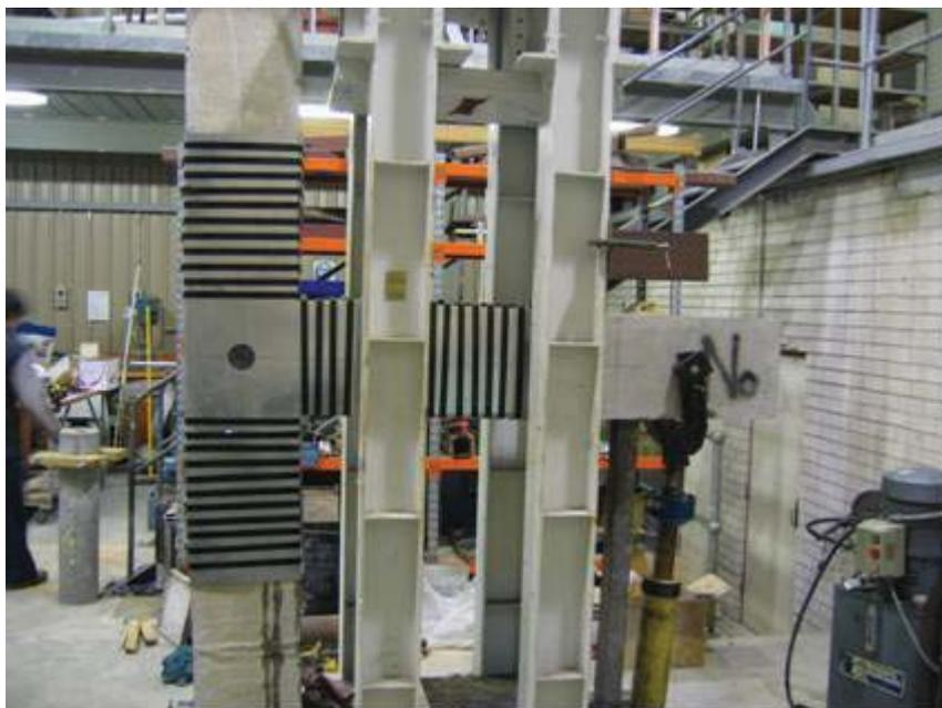
Figure 7 T-Connection completed with steel straps
