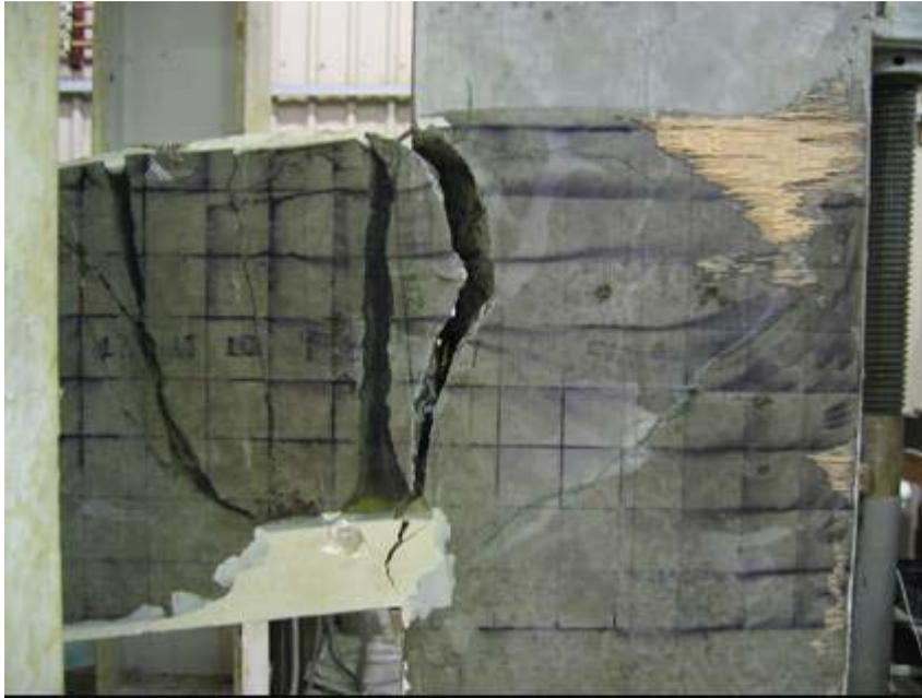
Figure 14 Rehabilitated specimen after testing
