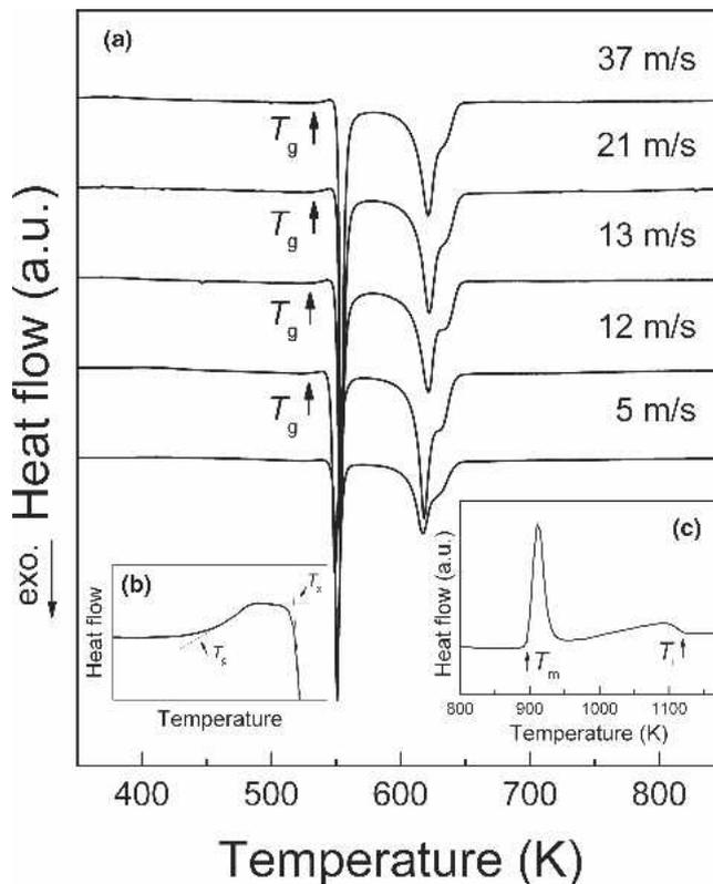
FIG. 3. (a) DSC scans of the melt-spun  $\text{Al}_{85}\text{Ni}_9\text{Nd}_4\text{Co}_2$  ribbons prepared at different wheel speeds (heating rate 40 K/min), (b) an enlarged view of a DSC trace near the glass transition, and (c) melting behavior of the as-spun ribbon prepared at 21 m/s (heating rate 20 K/min).
