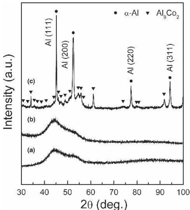
FIG. 6. XRD patterns of  $\text{Al}_{85}\text{Ni}_9\text{Nd}_4\text{Co}_2$  samples in different states: (a) as-spun glassy ribbon prepared at 21 m/s, (b) as-milled powder prepared by milling the as-spun ribbon (milling parameters: 200 rpm, 9 h), and (c) as-milled powder obtained by mechanical alloying of the elemental powders mixture (180 rpm, 140 h).
