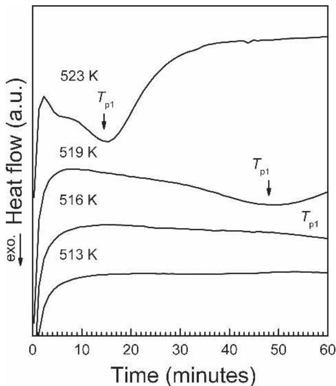
FIG 8. Isothermal DSC curves at different temperatures for the as-milled powder obtained by ball milling starting from the  $\text{Al}_{85}\text{Ni}_9\text{Nd}_4\text{Co}_2$  ribbon (21 m/s).
