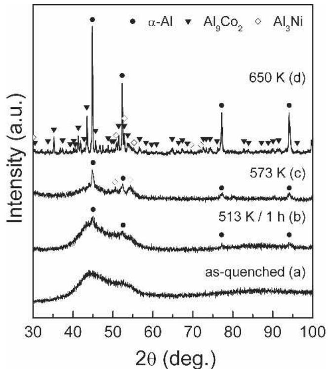
FIG. 5. XRD patterns measured at room temperature for the Al<sub>85</sub>Ni<sub>9</sub>Nd<sub>4</sub>Co<sub>2</sub> ribbon prepared at 21 m/s: (a) as-spun ribbon, (b) after isothermal annealing at 513 K for 1 h, (c) after the first crystallization event at 573 K, and (d) after the second crystallization event at 650 K obtained for the samples scanned in the DSC at a heating rate of 40 K/min.
