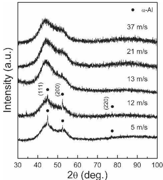
FIG. 1. XRD patterns of the melt-spun Al<sub>85</sub>Ni<sub>9</sub>Nd<sub>4</sub>Co<sub>2</sub> ribbons prepared at different wheel speeds.
