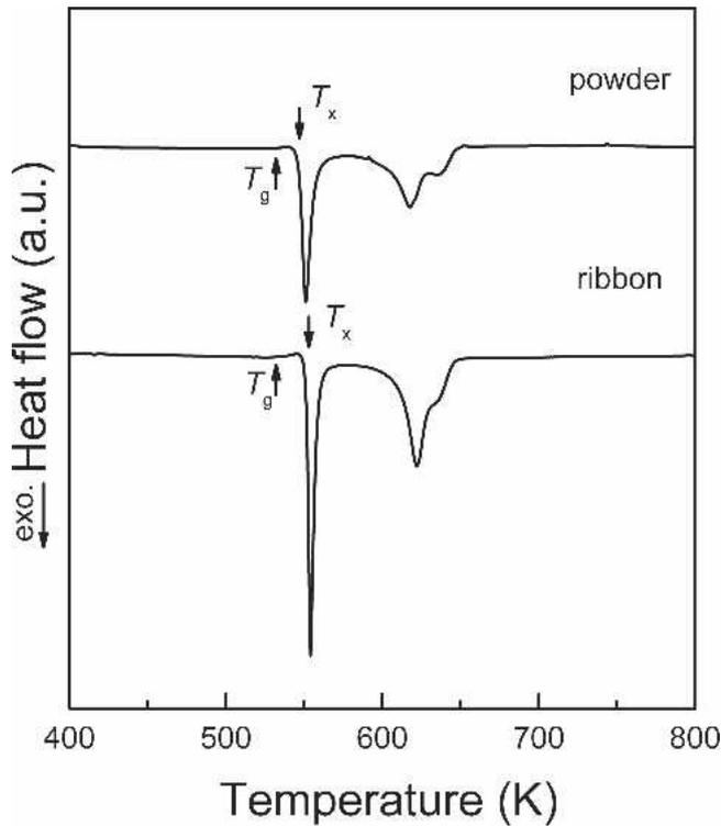
FIG 7. DSC scans of  $\text{Al}_{85}\text{Ni}_9\text{Nd}_4\text{Co}_2$  samples in different states: (a) as-spun glassy ribbon (21 m/s) and (b) as-milled powder (200 rpm, 9 h) prepared from the ribbon.
