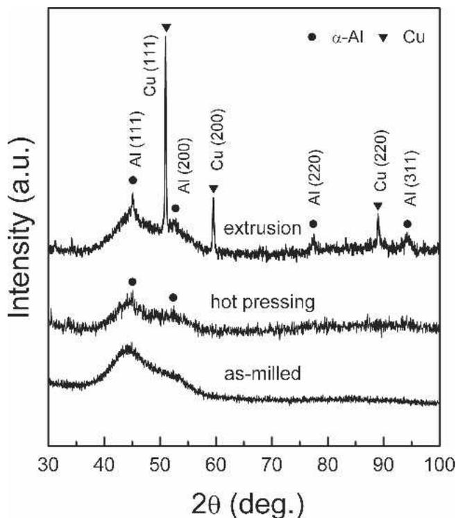
FIG 9. XRD patterns of (a) as-milled powder and bulk samples after consolidation via (b) uniaxial hot pressing and (c) extrusion for the  $\text{Al}_{85}\text{Ni}_9\text{Nd}_4\text{Co}_2$  alloy. (The Cu phase peaks stem from the Cu can used for encapsulation of the samples).
