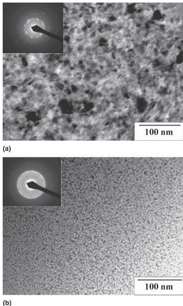
FIG. 2. TEM bright-field micrographs and the corresponding selected area diffraction patterns (inset) of the melt-spun  $\text{Al}_{85}\text{Ni}_9\text{Nd}_4\text{Co}_2$  ribbons prepared at (a) 5 m/s and (b) 21 m/s.
