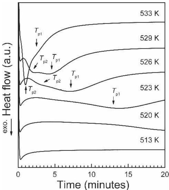
FIG. 4. Isothermal DSC curves recorded at different temperatures for the Al<sub>85</sub>Ni<sub>9</sub>Nd<sub>4</sub>Co<sub>2</sub> ribbon prepared at 21 m/s.
