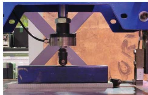
**Fig. 5b** Validation of shear force measurements
