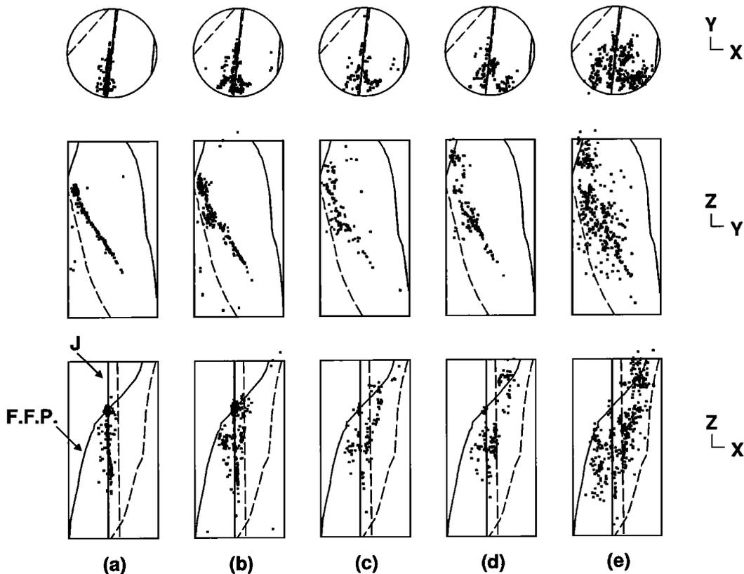
Figure 2. Orthographic projection showing the spatial distribution of AE hypocenters during (a) 0-60, (b) 60-100, (c) 100-110, (d) 110-113, and (e) 113-114 minutes from the beginning of creep. Surface traces of the final fracture plane (F.F.P.) and the pre-existing joint (J), which appeared on the front and rear sides of the sample, are drawn by solid and dashed lines, respectively.
