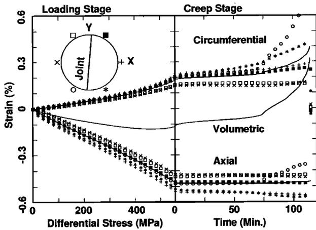
Figure 1. Strains as functions of differential stress during the loading stage (left) and of time during the creep stage (right). The solid lines indicate the average strains. Symbols indicate positions of the strain gauges.
