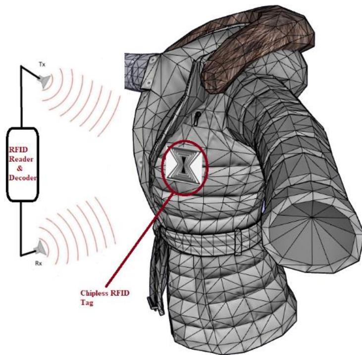
Figure 1: Structural diagram of Bow-Tie chip-less RFID system
