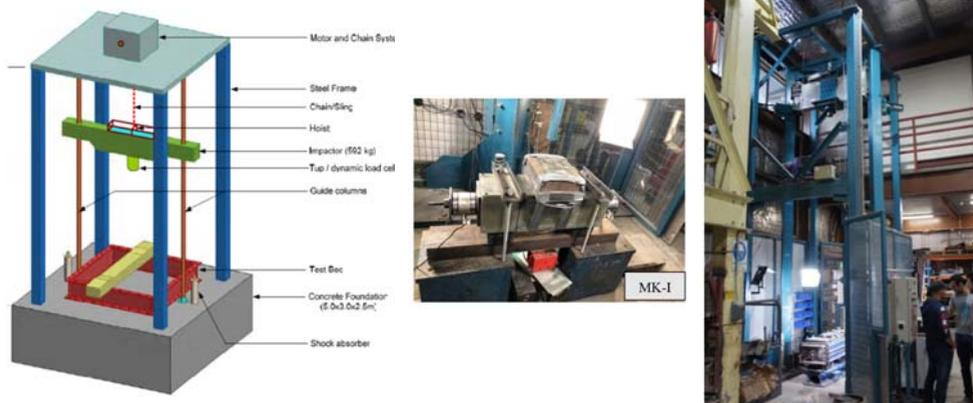
**Fig. 2.** Drop hammer test and MK-I set up
