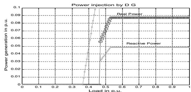
**Figure 8a:** Power generation by DG-QPQ (0.95 p.u. voltage threshold)
