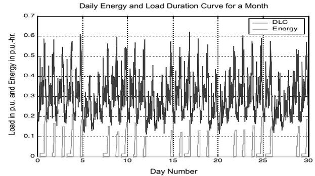
**Figure 11b:** Daily load demand and DG energy for a month with DG-QPQ (0.95 p.u. voltage threshold).
