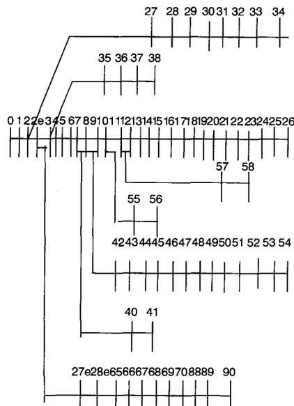
Fig. 3 Schematic diagram of 69-bus distribution system
