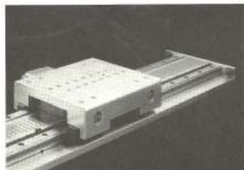
Figure 1: cage-secondary single-sided LIM (Photo Courtesy of Krauss Maffei Automationstechnik GmbH)
