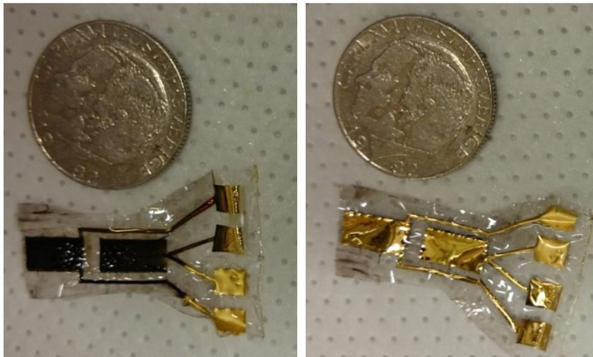
Fig 3. A photo graph of the finished trilayer microactuator device mimicking a finger that can be articulated. The device comprises two actuators that are  $5 \times 10 \text{ mm}^2$  each.
