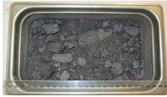
Figure 6 (d). Coalwash after 25 cycles of wetting and drying cycle.
