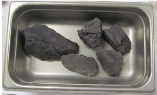
Figure 6(c). Coalwash before wetting and drying cycle.
