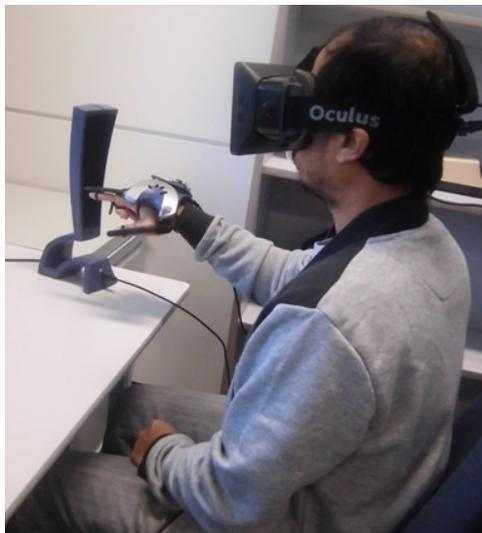
Figure 2. Operator with data glove and the feedback system.
