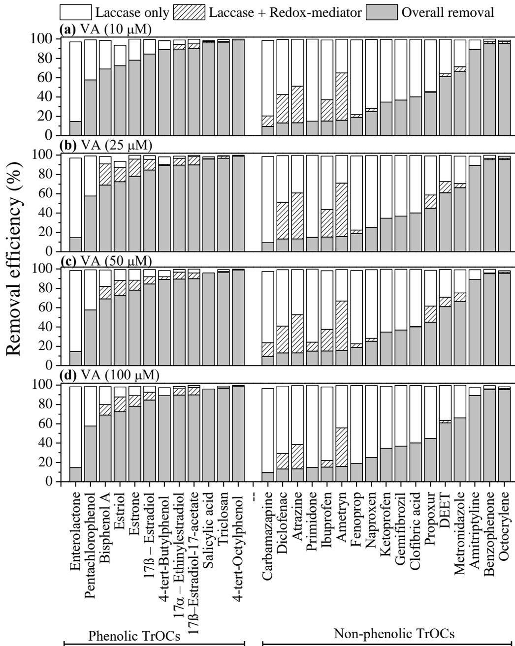
**Figure S6:** Improvement in TrOC degradation by adding single dose VA at different concentration separately at the start of NF-EMBR operation. VA showed compound-specific and concentration dependent improvement. The overall removal of TrOCs in NF-EMBR was >90%. The NF-EMBR were operated for a period of 68 h in continuous mode at an initial HRT of 16 h.
