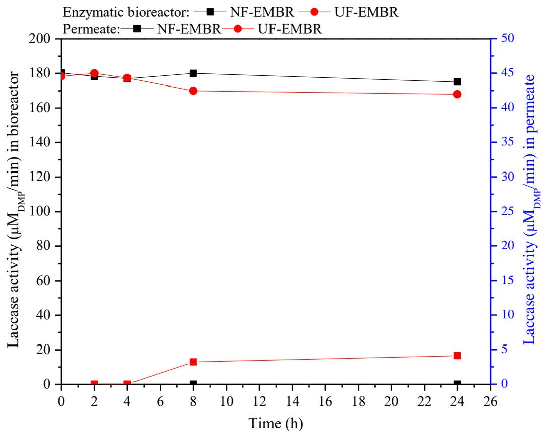
**Figure S2:** Confirmation of effective laccase retention by the NF and UF membrane. Laccase retention of >99% and 95% was achieved by the NF and UF membrane respectively. UF/NF-EMBR were operated for a period of 24 h in full recirculation mode without the addition of TrOCs.
