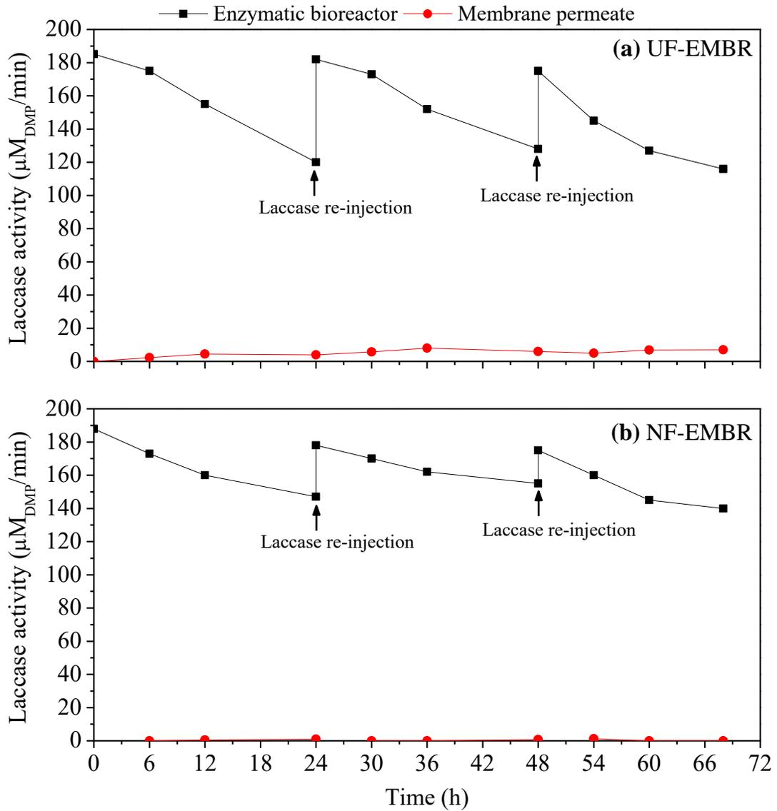
**Figure S3:** Laccase activity profiles in UF-EMBR (a) and NF-EMBR (b). Laccase activity was maintained by re-injecting a small dose of laccase (250  $\mu\text{L}$  per litre of bioreactor volume) every 24 h.
