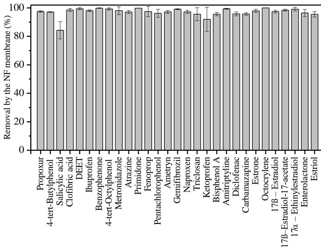
**Figure S4:** Removal of TrOC by the NF membrane to confirm their effective retention. NF-EMBR were operated for a period of 32 h in continuous mode without the addition of laccase. The UF-EMBR was not operated because the UF membrane was not expected to retain TrOCs. Data presented as average  $\pm$  standard deviation (n=2).
