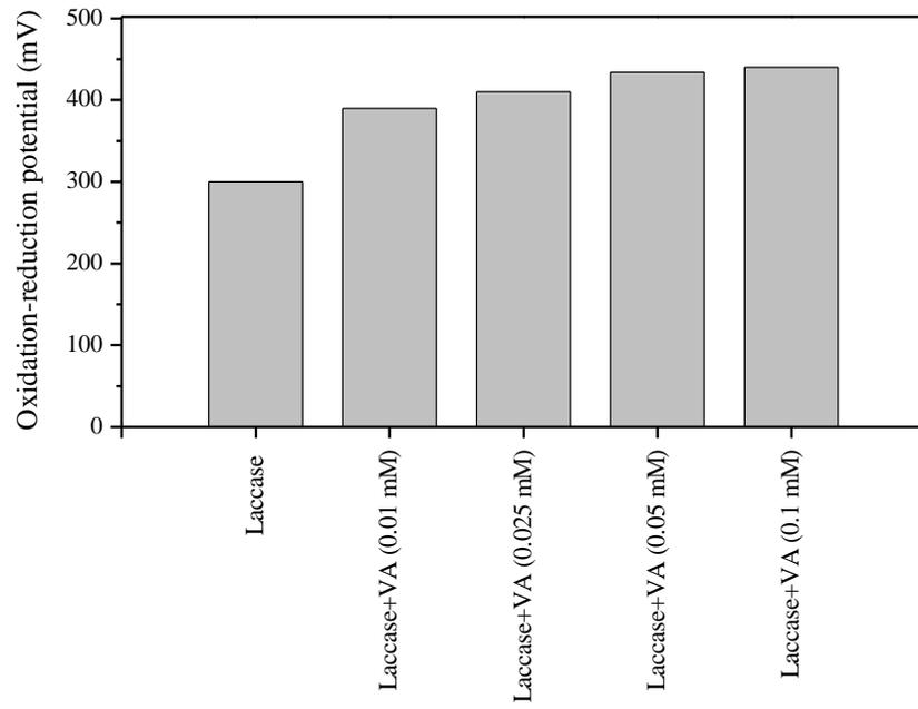
**Figure S5:** Impact of VA concentration on the oxidation reduction potential of media in NF-EMBR
