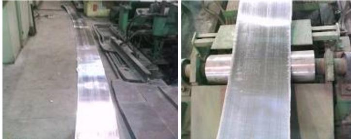
Fig. 2 5005 aluminum alloy sheet by roll-casting
