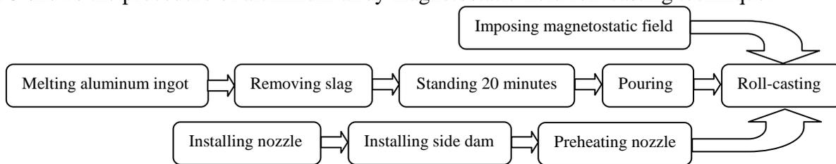
Fig. 3 The procedure of aluminum alloy magnetostatic field roll-casting technique
