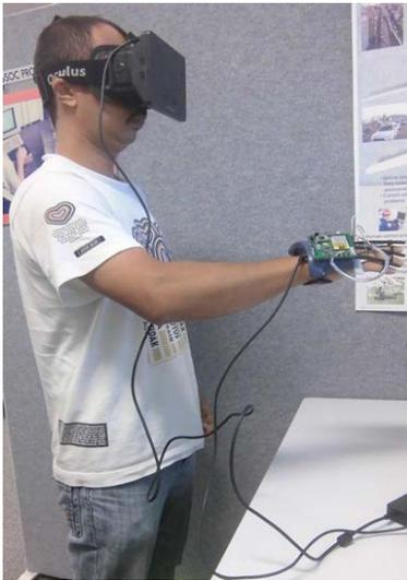
Figure 2. Operator with data glove and the feedback system.
