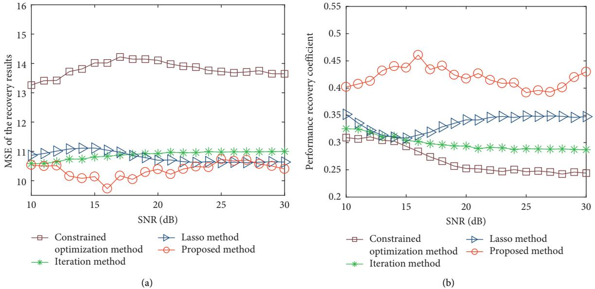
FIGURE 6: MSE and PRC of the sparse recovery results with the constrained optimization method [14], iterative method [15], Lasso method, and proposed method with different SNRs ( $M = N = 15$ ,  $\gamma = 15$ , and  $\rho = 0.2$ ). (a) MSE of the sparse recovery results with different SNRs. (b) PRC of the sparse recovery results with different SNRs.
