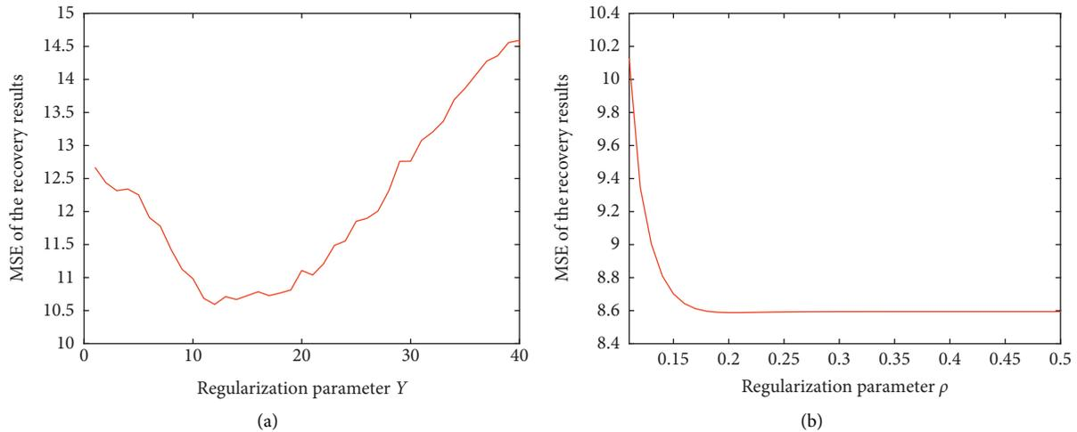
FIGURE 7: Effect of the regularization parameter  $\gamma$  and penalty parameter  $\rho$  on the MSE of the recovery results. (a) Convergent curve ( $\rho = 0.2$ ). (b) Convergent curve ( $\gamma = 15$ ).
