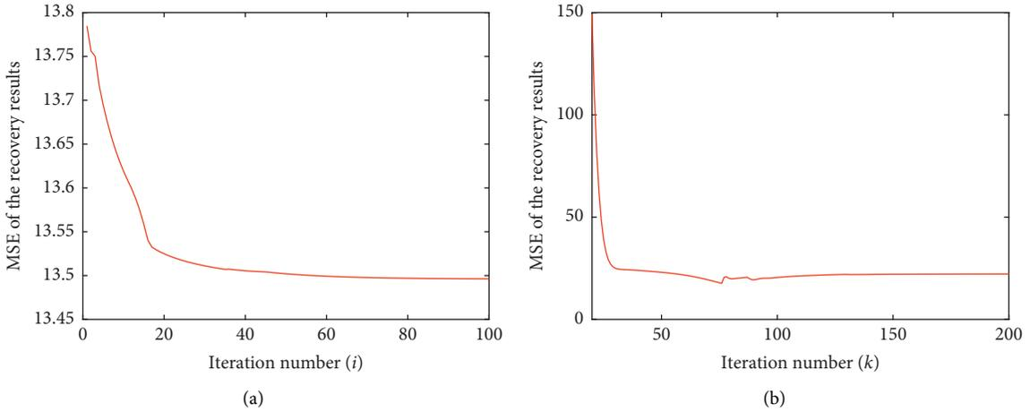
FIGURE 2: MSE of the reconstruction results with different numbers of iterations of  $i$  and  $k$  when  $M = N = 15$  and  $\text{SNR} = 20$  dB. (a) MSE with the iteration number  $i$  when  $k = 200$ . (b) MSE with the iteration number  $k$  when  $i = 60$ .
