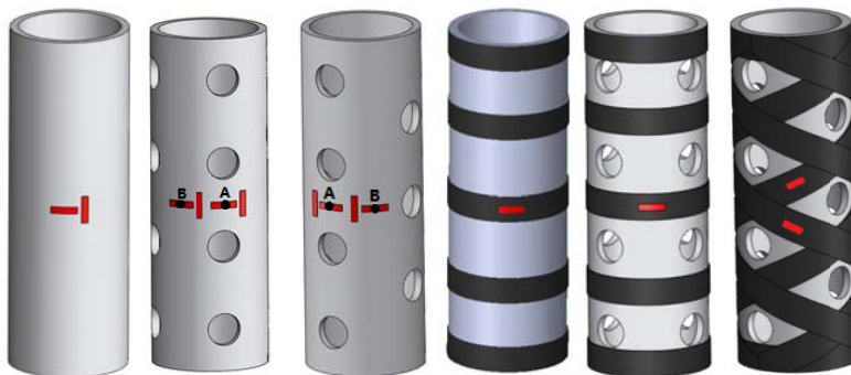
Fig. 8. Locations of strain gauges in GFRP tubes.
