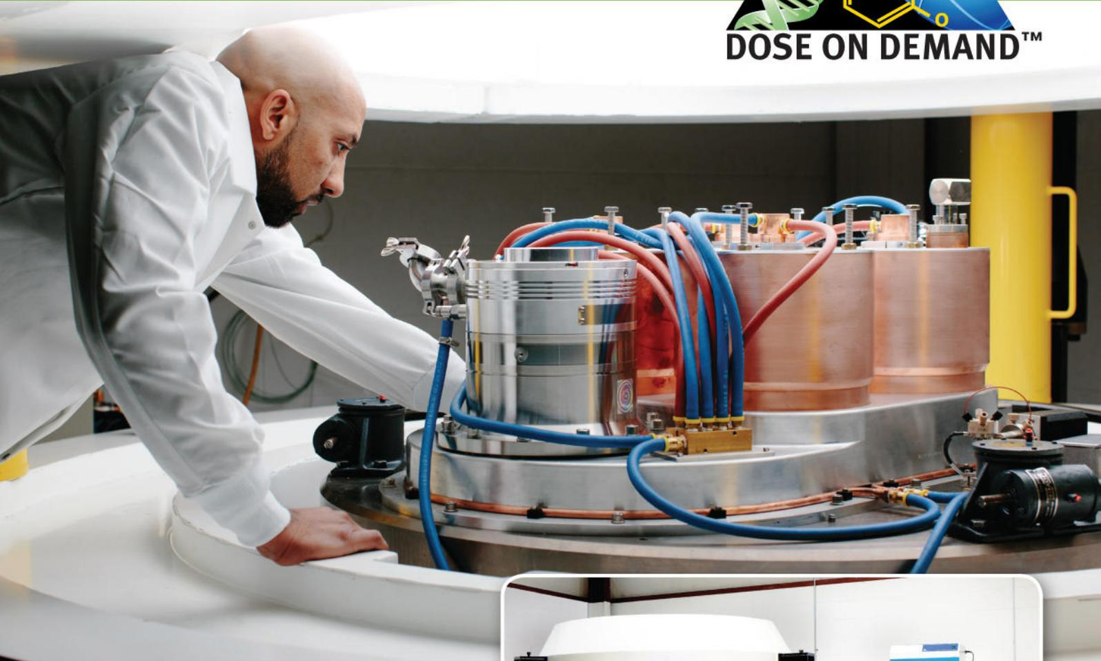
The BG-75 Biomarker Generator integrates a compact mini-cyclotron, kit based micro-chemistry, and automated quality control, simplifying in-house production of  $^{18}\text{F}$ -FDG and advanced biomarkers.
