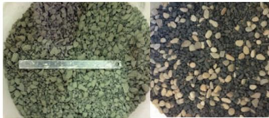
Figure 2. Gravel-sized Materials (M1 – left and M2 – right) used for Model Stone Columns
