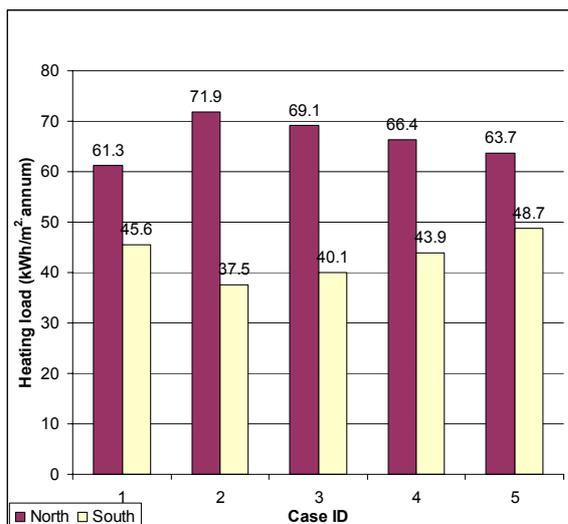
**Figure 6:** Comparison of heating loads according to window-to-wall ratios of no balcony options.
