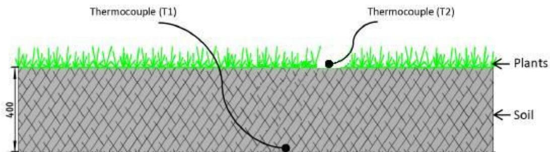
**Figure 2.** Cross sectional view of the green roof showing the position of the sensors
