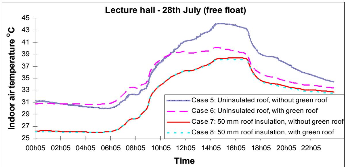
**Figure 10.** Sample of indoor air temperature improvements during the peak cooling season
