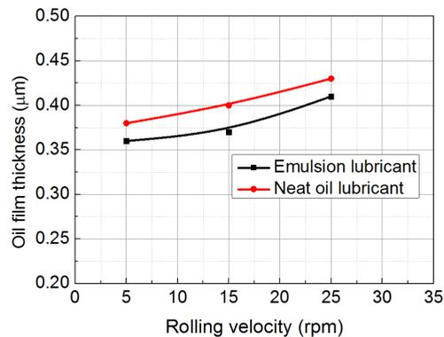
Fig. 6. Oil film thickness versus rolling velocity in experiment ( $H=100\ \mu\text{m}$ ;  $r=20\%$ ).
