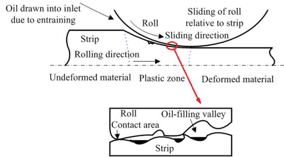
Fig. 2. Schematic of lubrication mechanisms in rolling.
