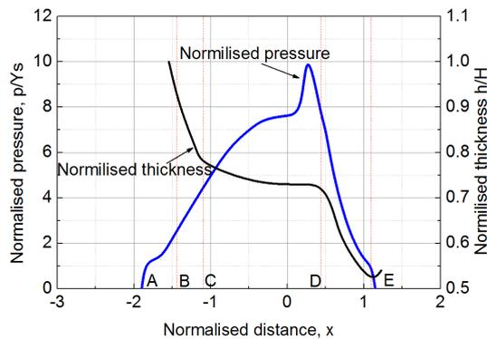
Fig. 4. Normalised thickness and pressure distribution for H=50µm, D=27 mm, µ=0.15, E<sub>R</sub>=580GPa.
