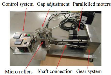
Fig. 1. Micro rolling mill with flexible speed ratio.
