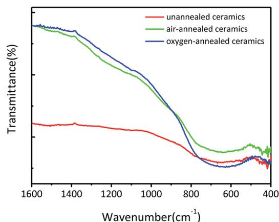
Fig. 3 FT-IR spectra of the obtained (Nb + In) co-doped TiO<sub>2</sub> ceramics.
