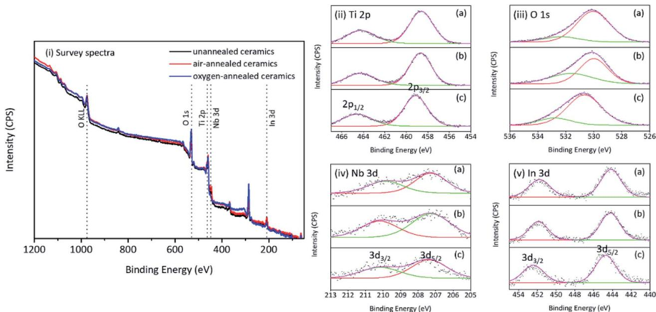
Fig. 4 (i) XPS survey spectra of as-prepared (Nb + In) co-doped  $\text{TiO}_2$  ceramics, (ii) the XPS spectra of Ti 2p band, (iii) the XPS spectra of O 1s band, (iv) The XPS spectra of In 3d band, (v) the XPS spectra of Nb 3d band for un-annealed ceramics (a), air-annealed ceramics (b) and oxygen-annealed ceramics (c).
