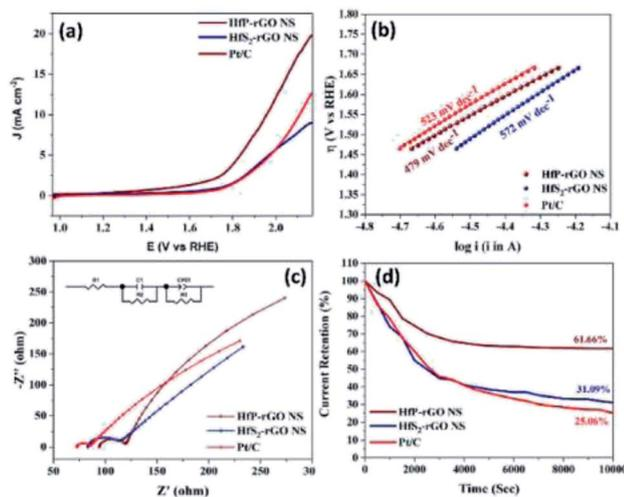
Fig. 7 (a) OER polarization curves in 0.1 M KOH solution at a sweeping rate of  $5 \text{ mV s}^{-1}$  (rotation: 1600 rpm), (b) Tafel plots, (c) Nyquist plots with corresponding equivalent circuit (inset) and (d) amperometric  $i-t$  test results of HfP-rGO and HfS<sub>2</sub>-rGO nanosheets.
