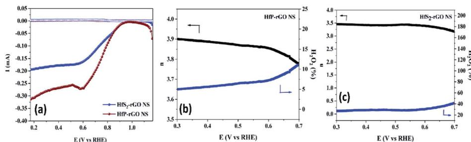
Fig. 6 (a) Rotating ring-disk electrode voltammograms of HfP-rGO NS and HfS<sub>2</sub>-rGO NS. Electron transfer number ' $n$ ' and H<sub>2</sub>O<sub>2</sub>% production for (b) HfP-rGO NS and (c) HfS<sub>2</sub>-rGO NS.
