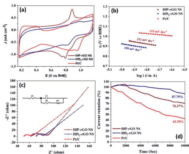
Fig. 4 ORR electrochemical measurements of HfP-rGO and HfS<sub>2</sub>-rGO nanosheets: (a) cyclic voltammograms in O<sub>2</sub> saturated 0.1 M KOH solution at a sweeping rate of 20 mV s<sup>-1</sup>, (b) Tafel plots, (c) Nyquist plots with corresponding equivalent circuits (inset) and (d) amperometric *i*-*t* curve studies.
