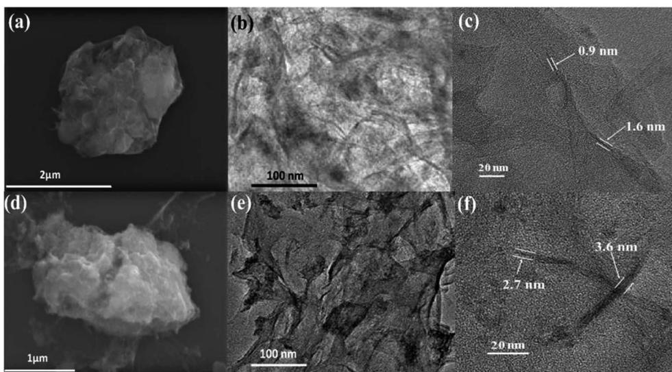
Fig. 3 (a) SEM, (b) TEM and (c) HRTEM image of HfP-rGO nanosheets. (d) SEM, (e) TEM and (f) HRTEM image of HfS<sub>2</sub>-rGO nanosheets.
