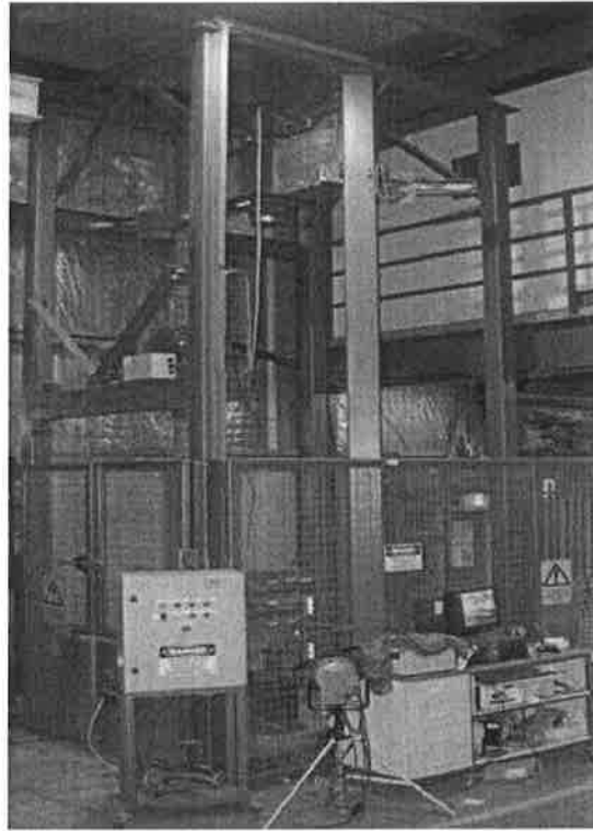
Figure 7: Drop weight impact testing equipment.
