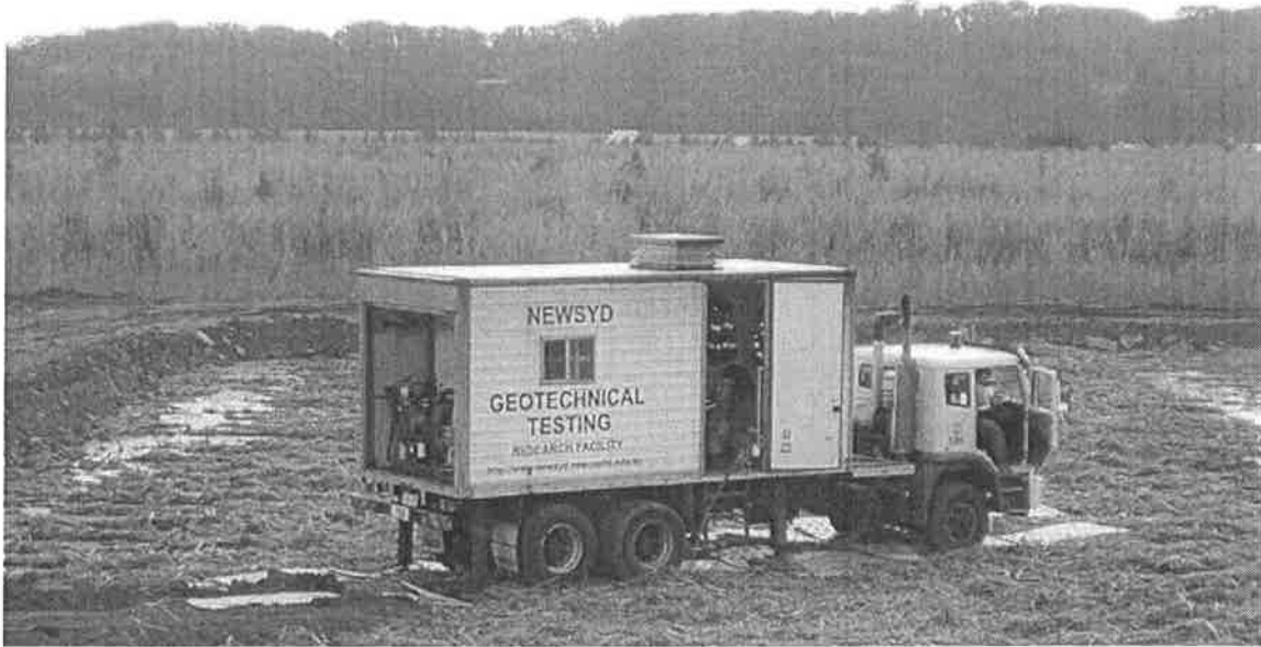
Figure 4: Current NewSyd facility at the Ballina site. Note the temporary working platform to support the vehicle weight.
