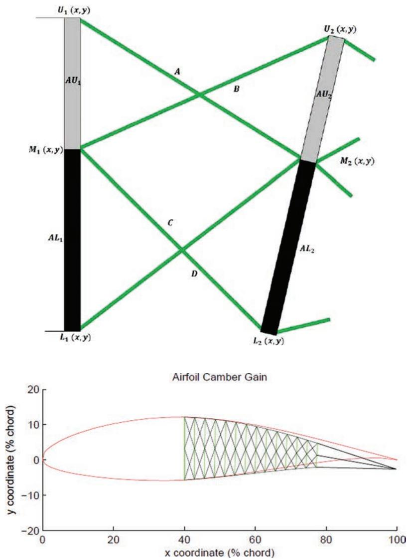
Figure 3. (a) One element of the compliant mechanism is shown; the nomenclature used in the following kinematic analysis is displayed (b) Airfoil with 14 actuator stacks spaced at 2.88% chord intervals starting at the 40% chord, a negative TE deflection of 2.62% chord is observed
