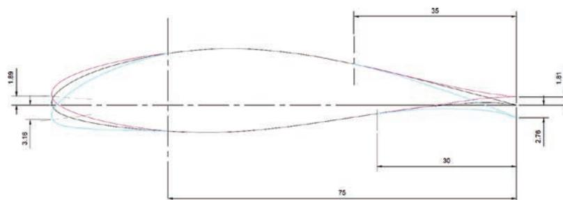
Figure 1. The required profile deformation (in % chord units) to achieve  $\Delta C_L \pm 0.4$
