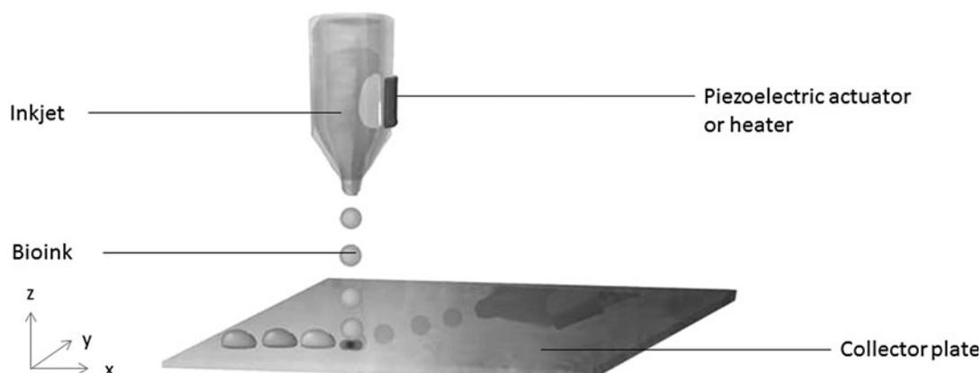
**Figure 2.** Schematic representation of an inkjet printer.
