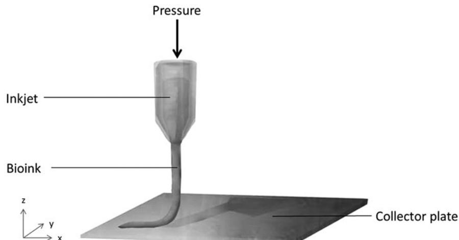
**Figure 4.** A schematic representation of an extrusion printer.
