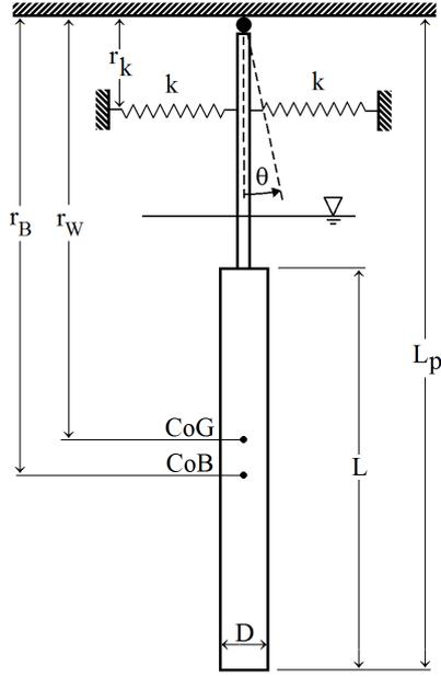
Figure 2 Experimental apparatus and parameter definition sketch.
