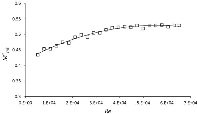
Figure 5. Pivoted-system critical-point variation with flow Reynolds number.
