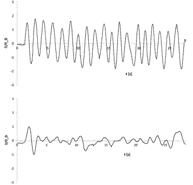
Figure 3. Time response above (a)  $M^*=0.33$  and below (b)  $M^*=0.70$  the critical point:  $Re=1.2 \times 10^4$ .
