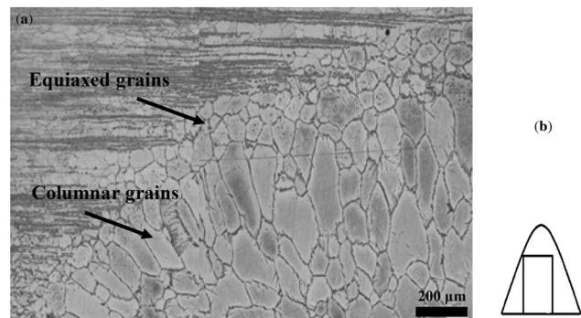
**Figure 4.** Microstructure of the unstabilised ferritic stainless steel (A:0Ti;0Nb) at 2% strain and welding speed of 3 mm/s showing (a) the base metal, HAZ region and the weld centre and (b) schematic orientation of the micrographs with respect to the fusion zone.
