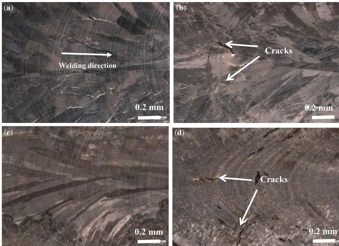
**Figure 2.** Typical stereoscopic images showing (a) alloy A:0Ti;0Nb with no crack at a welding speed of 3 mm/s and strain 1%, (b) solidification cracks in the B:0.6Nb-stabilised ferritic stainless steel at a welding speed of 6 mm/s and 2% strain, (c) alloy C:0.1Ti;0.4Nb with no crack at a welding speed of 3 mm/s and 1% strain and (d) solidification cracks in alloy D:0.4Ti;0.9Nb at a welding speed of 6 mm/s and 2% strain ( $\times 25$ ). For all four images, the welding direction was as shown.
