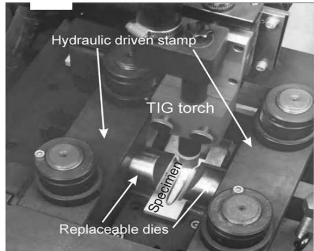
**Figure 1.** Example of the MVT test equipment [19].
