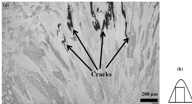
**Figure 6.** Microstructure of the 0.4Ti + 0.9Nb-stabilised ferritic stainless steel (D:0.4Ti;0.9Nb) at 4% strain showing (a) the base metal, HAZ region and the weld centre at a welding speed of 3 mm/s and (b) schematic orientation of the micrographs with respect to the fusion.
