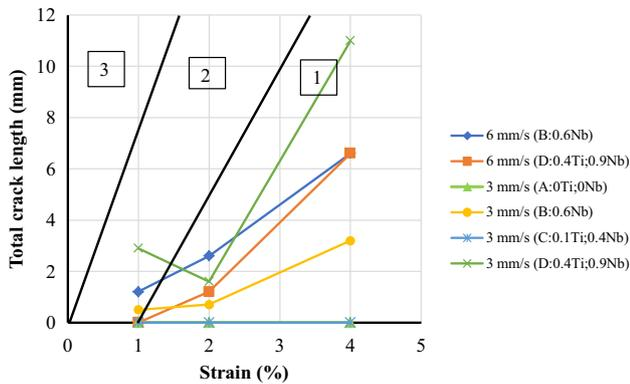
**Figure 3.** Total crack length vs strain for the welding speeds of 6 and 3 mm/s (BAM). Region 1: hot crack resistant, Region 2: increasing hot cracking susceptibility, Region 3: hot crack-prone. Every data point represents the total crack length on one sample.
