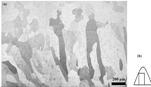
**Figure 5.** Microstructure of the 0.6Nb-stabilised ferritic stainless steel (B:0.6Nb) at 2% strain and welding speed of 6 mm/s showing (a) the base metal, HAZ region and the weld centre and (b) schematic orientation of the micrographs with respect to the fusion.
