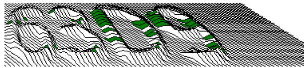
Figure 14: Extracting key features based on changes in line direction.
