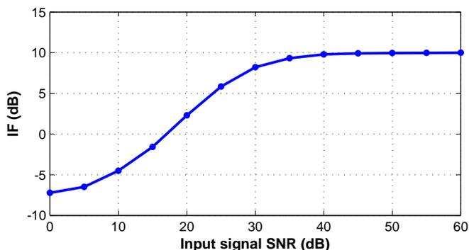
Fig. 11. Improvement factor of the image as a function of the SNR of the input radar signal.
