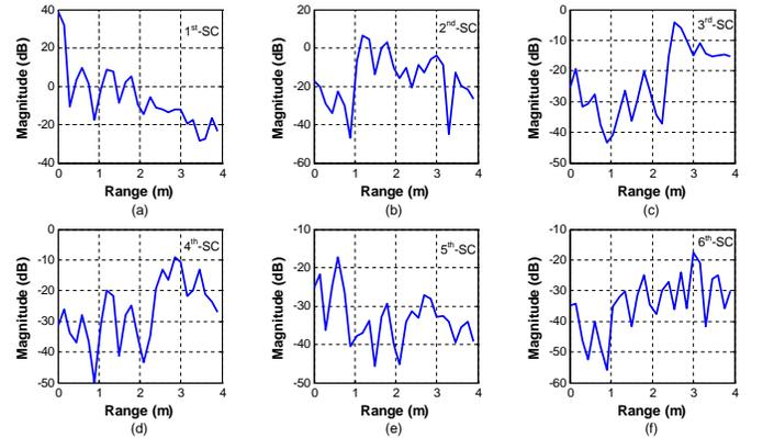
Fig. 8. The range profiles of the first 6 dominant singular components (1<sup>st</sup>-SC to 6<sup>th</sup>-SC).
