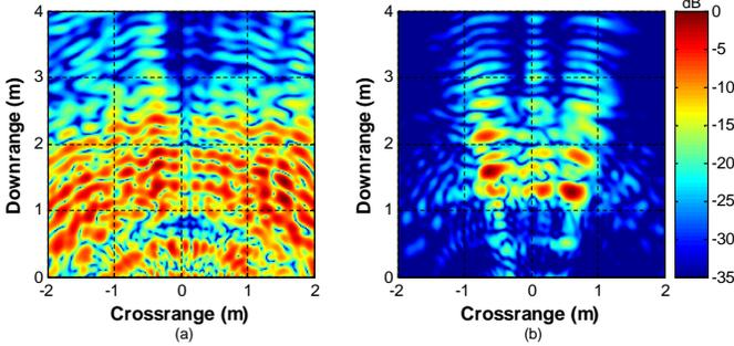
Fig. 9. Images formed using a subset of singular components: (a) image obtained from the 5<sup>th</sup>-SC only and (b) image obtained from the combination of these singular components: 3<sup>rd</sup>-SC, 4<sup>th</sup>-SC, and 6<sup>th</sup>-SC.
