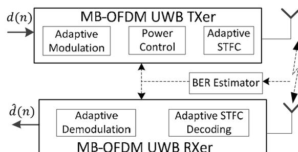
Figure 1 Adaptive STFC MB-OFDM UWB WBAN.
