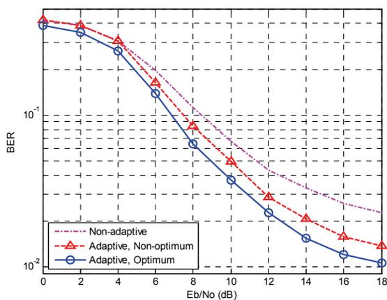
**Figure 3** Optimal adaptive and non-optimal adaptive performances in a  $2 \times 1$  MIMO configuration.
