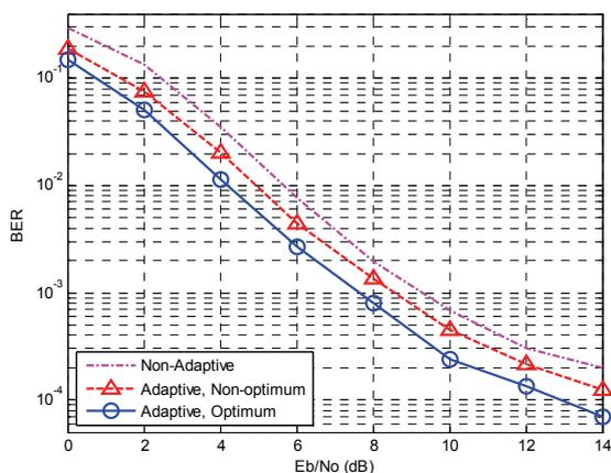
**Figure 4** Optimal adaptive and non-optimal adaptive performances in a  $2 \times 2$  MIMO configuration.
