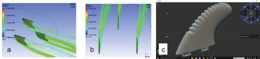
**Figure 4.** a) and b) Screenshots of computational fluid dynamics simulation of fins in an idealized surfboard under a yaw angle of 15 degrees. c) Screenshot of a computer aided design with bumpy leading edges on our fin design.
