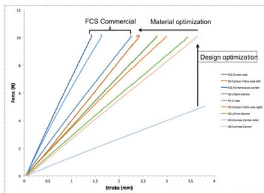
**Figure 3.** Applied force as a function of stroke of the experimental 3D printed and control surfboard fins tested under laboratory conditions. Vertical arrow, horizontal arrow and “FCS Commercial” indicate optimization of 3D printed fin designs, material optimization and commercial fins as manufactured by FCS.
