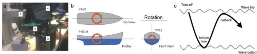
**Figure 1.** a) Photograph of the setup used to characterise the fins under laboratory conditions, numbers 1-4 indicate mechanical analyzer, fin, rig to clamp fin and computer for data collection, respectively. b) Schematic representation of the three rotational angles of a surfboard, yaw, pitch and roll. c) Schematic representation of the path of a surfer on a typical wave going from take-off via a bottom turn into a cutback.
