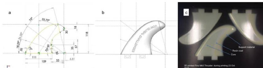
**Figure 2.** a) Screenshot of computer aided design (CAD) of fin. Numbers indicated parameters that can be varied in the design. b) CAD image showing lateral aspect of the fins c) Photo of typical 3D printed thruster fin set during printing on a Objet Connex printer.
