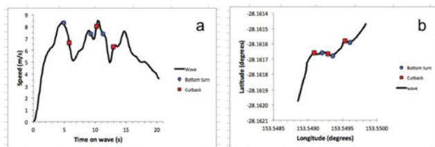
**Figure 5.** Examples data of Participant 2 riding a surfboard with 3D printed fins (ULTEM) in a thruster configuration on a typical wave (Snapper Rocks, Australia): a) Speed versus time. b) GPS data. Circles and squares indicate bottom turns and cutbacks, respectively.
