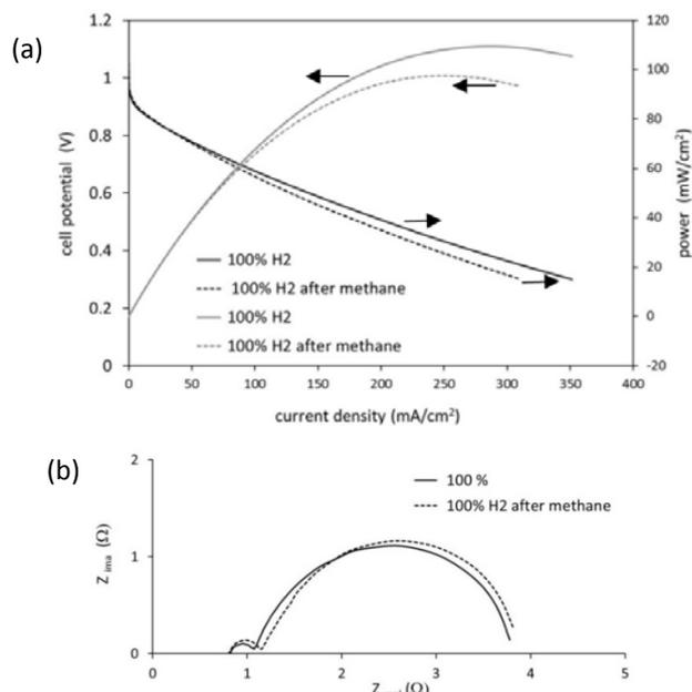
**Figure 7.** (j-V), (j-P) (a) and GEIS at 10 mA/cm<sup>2</sup>, (b) characteristics for a fuel cell operating with pure hydrogen before (solid lines, black for j-V and grey for j-P) and after measurements with hydrogen and methane mixtures.
