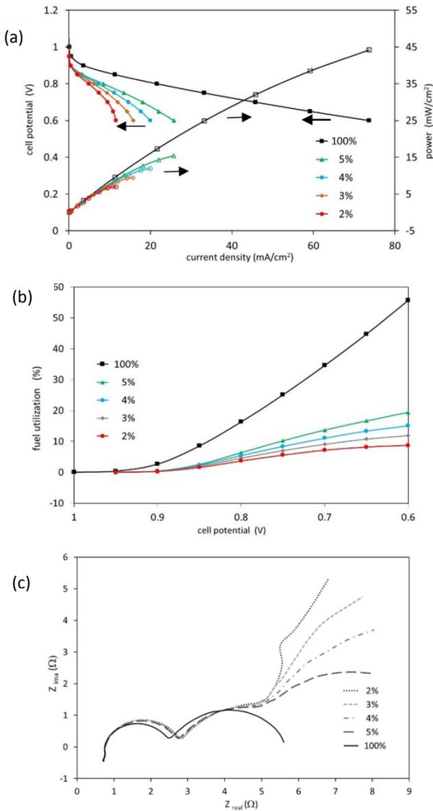
**Figure 8.** (a) (j-V) and (j-P) characteristics, (b) fuel utilization, and (c) galvanostatic EIS at 10 mA/cm<sup>2</sup> for the cell (1 cm<sup>2</sup>) operating with: 100%, 5%, 4%, 3% and 2% hydrogen in the gas mixture.
