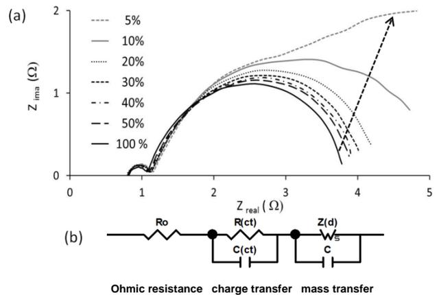
**Figure 6.** Nyquist spectrum of impedance measurements for cell (1 cm<sup>2</sup>) supplied with pure hydrogen and 50%, 40%, 30%, 20%, 10%, and 5% hydrogen and methane mixture. (a) The total flow was kept constant at 20 ml/min, constant current density of 10 mA/cm<sup>2</sup> was applied; (b) the equivalent circuit.
