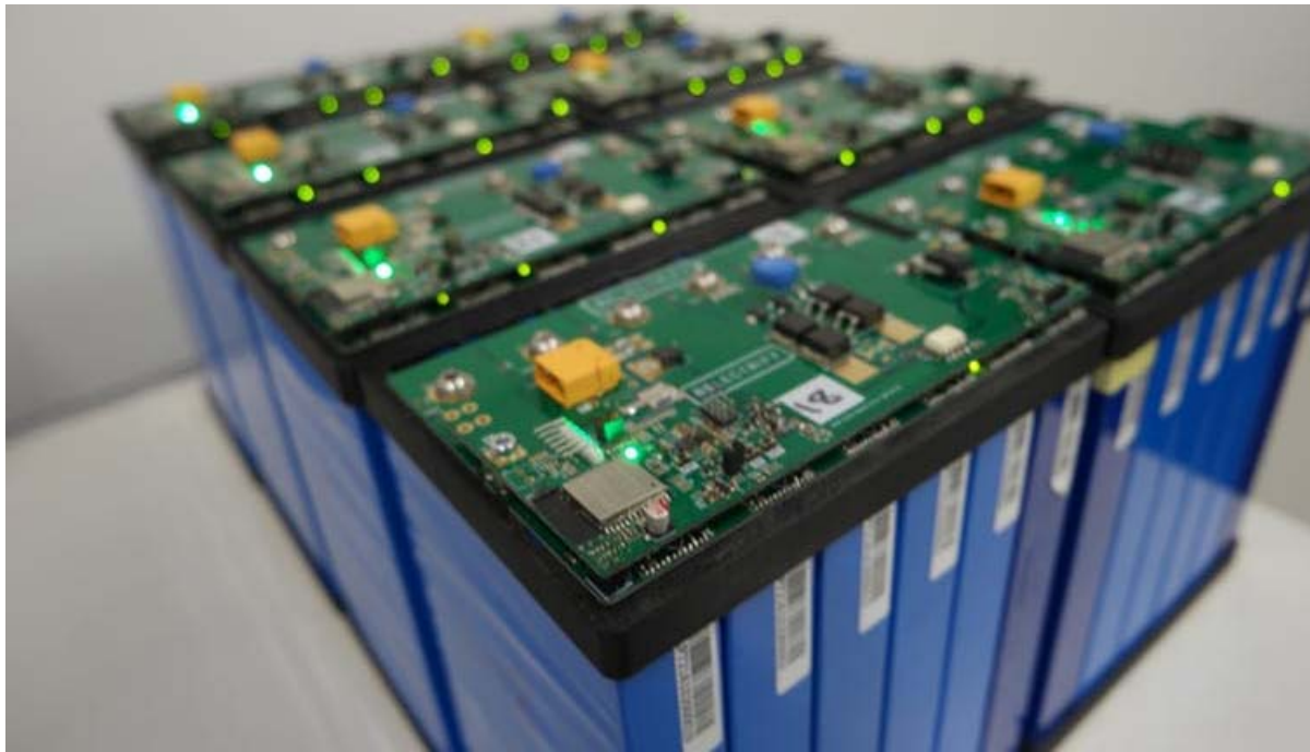
Relectrify's smart battery management system. from Relectrify
