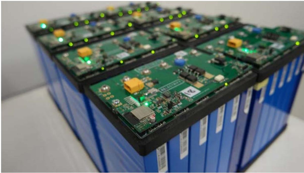
Relectrify's smart battery management system. from Relectrify
